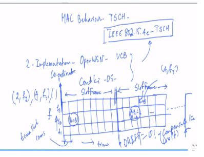
The MAC behavior of interest to us for several industrial applications is the time synchronized channel hopping MAC which is nothing but 802, so let us put it technically correct IEEE 802.15.4e-TSCH. You must not forget this because you can have dash DSME. You can have LLDN so on, right? So we are only worried about the TSCH implementation. Now as I mentioned to you the main implementation of this MAC, TSCH MAC is not a straightforward thing.
