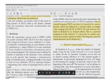
Now come to channel hopping. Now channel hopping is simple expression here. You can see that the frequency of interest is essentially a function of ASN. This is called the absolute slot number. Now what is absolute slot number? ASN simply means when the system was switched on, the coordinator sent out the first slot frame at this point.
