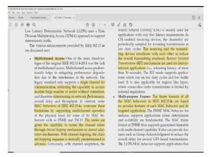
First one is multichannel access, okay. See the problem with the ZigBee system which we studied, there is one problem that you only have a single channel for your complete PAN system that you set up, okay. You have a PAN coordinator and all nodes identify the PAN coordinator and then they communicate to that PAN coordinator.
