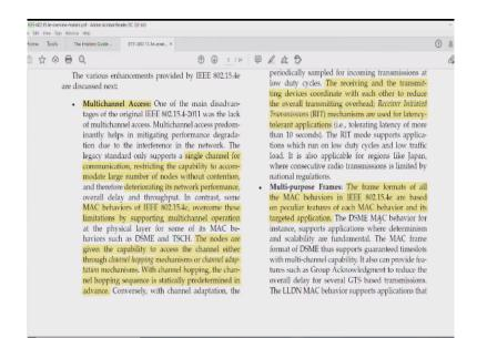
Then there is the third one, which is multi-purpose frames. Basically the advantage here is the frame formats of all MAC behaviors are based on the peculiar features of this MAC behavior and its targeted applications. So it is another important feature. You are not just configuring one type of frame, but you will be able to embed different MAC behaviors into that frame itself.
