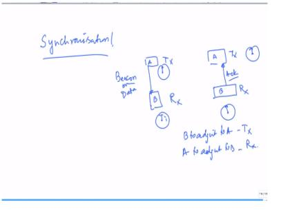
Synchronization is the key here and you can either do, you have a transmitter, you have a receiver. You either transmit. Whenever there is a Beacon, whenever there is a Beacon transmission the receiver can adjust its clock okay, exactly aligning to the transmitter's clock. Either you can do it with Beacon or you can also do it the other way, right. You can have, you have one clock here.
