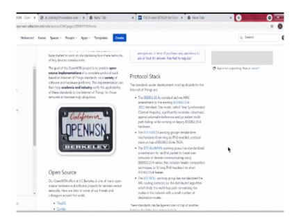
As mentioned here 15.4e standard defines the MAC and all that it writes. It says time synchronize channel hopping is there. And then this has been implemented. There is something called an IETF TSCH, 6TSCH working group, which is talking about how to have IPv6, running over time synchronized channel hopping.
