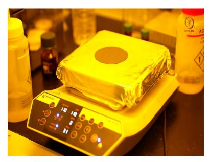
Another wafer is right. So the next step is to hot bake the wafer for three minutes at 110 degree Celsius, the hot baking step will harden the photoresist that remains so that it can sustain the metal deposition process that is going to happen next. Now the hot bake is complete. I am taking out the wafer, and now the wafer is ready for metal deposition.
