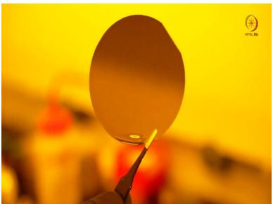
So now I am pouring the solution named as developers. So developer is the solution, which removes the soft photoresist, as I told you before, so and then we also have another petri dish with DI water. So after, so the development is time dependent. If you keep it in developer or wafer in developer for a long time, the required photoresist also will get removed, or the hard photoresist will also get removed.
