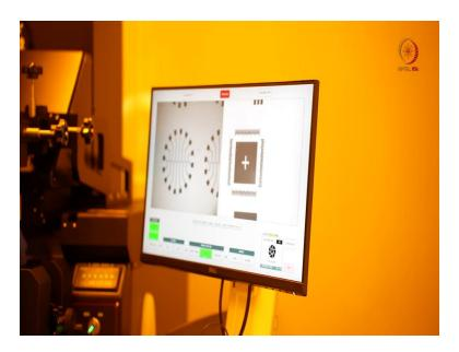
So this is the PC that controls the Mask Aligner, so I am switching it on, then followed by the power supply for the UV lamp ultraviolet lamp and fixing that as well on Now, we need to switch on the lamp power supply as well here. So when I proceed you can see some numbers written here, which corresponds to the current rating, voltage rating and the power. So now that the lamp is on we are going to switch on the equipment, so now the equipment is initializing.
