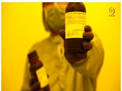
So I told you there are positive and negative photoresist, and this is an example of a positive photoresist, which is AZ 4562, this is a positive photoresist and what, most of the photoresist this number like this a 4562 has something associated with this number 4562 has something associated with this properties. So what it means is that the coating procedure or the spin coating procedure that we use for this photoresist is somewhat evident from this number.
