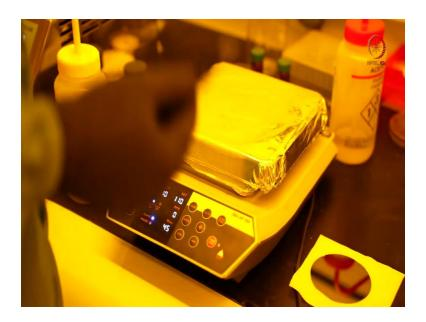
So now I will keep the wafer onto the hot plate. So the wafer is being kept at 110 degrees Celsius for one minute. So this process is known as soft bake. So I am taking out the wafer, it is been one minute. Now the next step is development.
