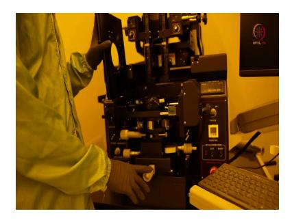
So what we have here is the Mask Aligner equipment, the name suggests Mask Aligner. So that means, the photomask that we have with the pattern can be aligned with the wafer or substrate in which we have the photoresist. So it is an alignment process. Now, we have the UV source Ultraviolent source that is within this chamber. So this is the UV source that is used to expose the photoresist 365 nanometer. Then we also have a microscope which we use for alignment.
