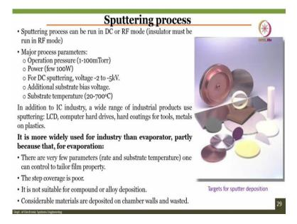
So, if you want to see in a glance by this sputtering process, then sputtering process can be run in DC or RF mode, the insulator must be done in RF mode is important. Then what is the second thing the major parameter process or process parameters are one operational pressure 1 to 100 milli Torr. Second the power it should be fewer than 100 Watts, we can also change the power actually in sputtering from 100 to 200 to 300 watts.
