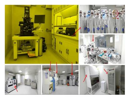
So, if you see the screen, this is the yellow room that is there in the screen which is a photolithography unit. And then there is a spin coding unit if you can see the screen so you have this yellow room. The reason of using yellow room is that you cannot expose the photoresist, so we use for this everything I will teach you, do not worry, there is something called photoresist.
