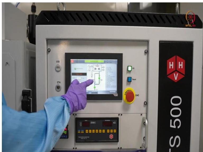
See, now it switched to fine pumping. Fine pumping means through the backing line, now it is getting pumped or evacuated by the turbomolecular pump. Just for a confirmation, you can
