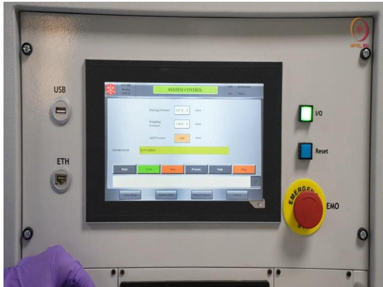
So, let us come here. So, here we are in system control window, in this monitor you can see, either you can start or you can vent. There is no point of venting because already the chamber is in atmospheric pressure, as we just loaded. And we can see here backing pressure is still lesser than atmospheric pressure because we are not, I mean, we did not open those valves.
