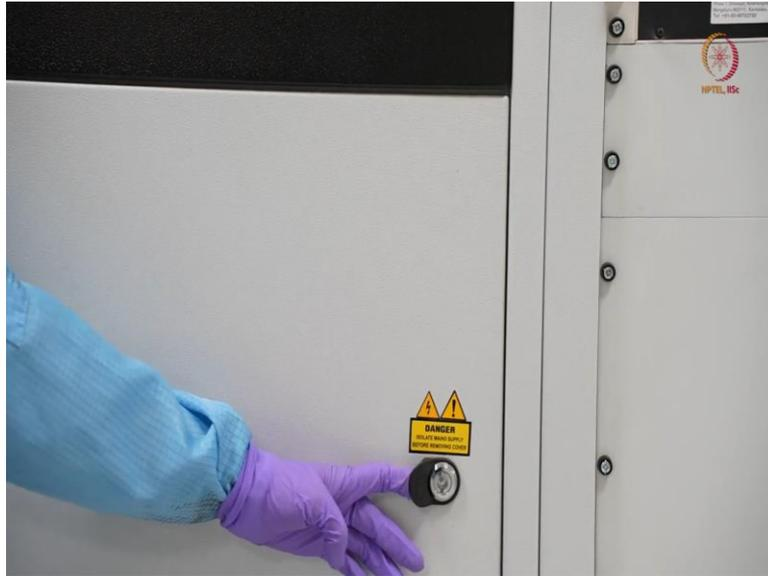
So, let us open this up. Before opening, you can just see here, before opening the door, you can see here again the similar warning again like electrical hazard that isolate main supply before removing this. So isolate main supply is better, whenever it is switched off, you can open this. It is not like you cannot open this when it is in action or when it is running, because this is a mechanical key.
