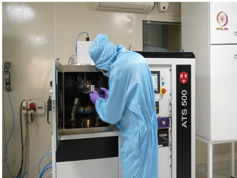
So we have the chuck here. We will just place it. This is the same process. So, closer view is not that important. So you have checked already during EBM evaporation. Similar loading process. So here when we are loading it, as we will be depositing in rotation, so it does not matter where we are actually loading the sample.
