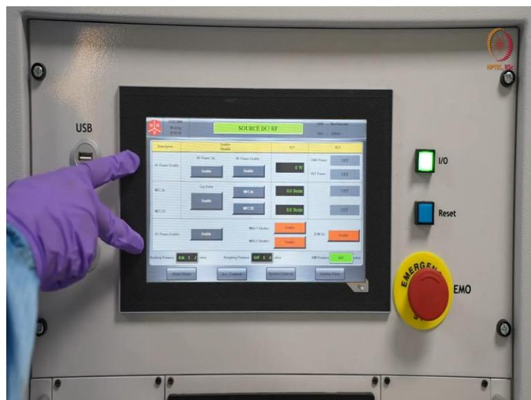
The source control as I already discussed, it will have all the information about this magnetron like RF power, DC power, these are two magnetrons, and this MFC or the mass flow controller, you can control how much gas will be flowing. And here magnetron shutter, whether to close or how to close, open, everything is here.
