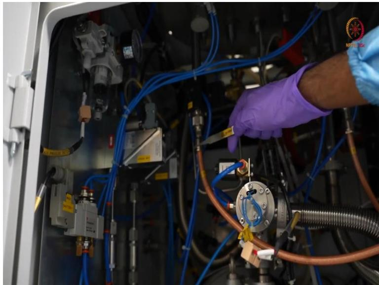
Then here you can see MFCs. So, argon MFC, you can see behind this, there is an oxygen MFC, MFC is Mass Flow Controller. So, what it does? So, we usually connect the gas pipelines to these and this will check as per the instructions given by you through the display or the interactive display basically.
