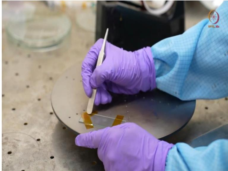
So here, you can see that normal blast slide I have just pasted one. So now, we will fix it with Kapton tape and in a single go we will deposit both the materials. Because here we are not actually targeting any particular device to fabricate. So, deposition is not, I mean deposition is important for demonstration purpose only.
