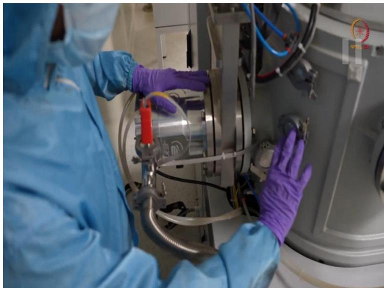
Here is one more penning gauge and this can, I mean and you can see this connection is through that. So, this is one of the backing lines, here, that you can see through this pump and this gauge, this is the backing gauge. So, here you can, here if you can see there are many ports that is possible, we can just attach some new parts to this. Now we will check it. We can check these things.
