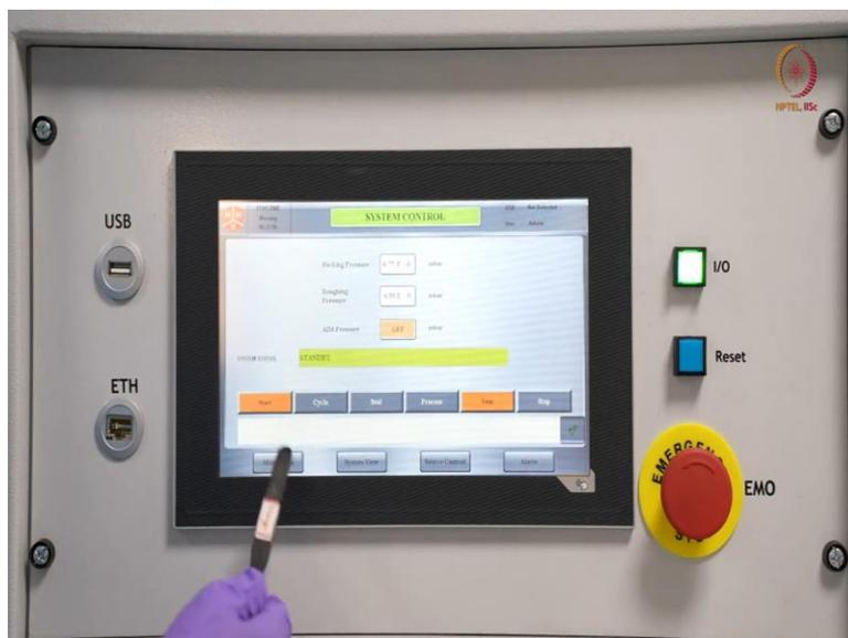
See, here it already sensed because during demonstration I pressed that emergency stop once and though I just released it, still it is showing that emergency stop placed. So, it is sensing that, that whatever happened to the tool. Here will just accept that error. So, whatever error will be there, that will be here, that will be shown here.
