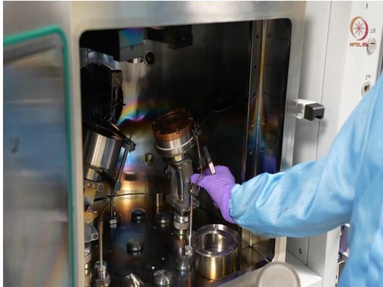
So, here actually you can see, this is the backplate is copper and here is the target. As we have used this earlier, so you can see that outside area that is still shiny and inside it is a little rough, because materials from here is already scraped out and it was deposited. So, with time there will be grooves. So, that will be visible. This is a new target. So, we cannot see that now only. But here you can see this is the magnetron so here we will get the negative connection.
