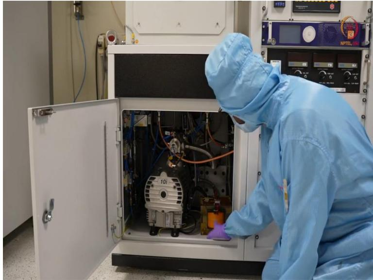
So, here if you can see, this is the same pump, rotary pump that we checked, when we have demonstrated that EBM evaporator system. This is the similar pump. So, here, it can go up to 10 power minus 4 or better to say 10 power minus 3 to 10 power minus 4 milibar range, as we have discussed earlier. And here, we have one transformer at the right side, here if you can see. So, that is to facilitate power to the system.
