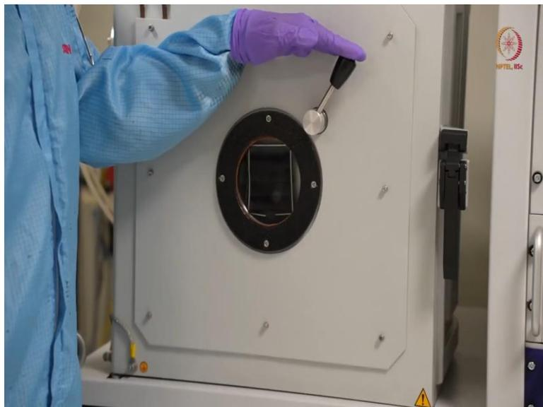
Starting with the components like this is the first one. So, this is the chamber. In operation tool also you have seen the similar chamber, but here you can see, I mean, here are the water flows that is required. So, inlet and outlet. Inlet water with, I mean from a chiller basically that is chiller outlet is inlet here.
