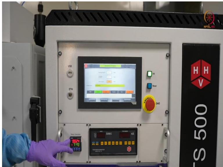
So, here actually you can see this can, this is showing now the chamber condition. So, like see this is 24, whatever it is in red that is basically whatever it is the temperature sensed by the temperature sensor placed inside just on above the check. So, in the chamber, where our sample is loaded, that temperature is 24 now.
