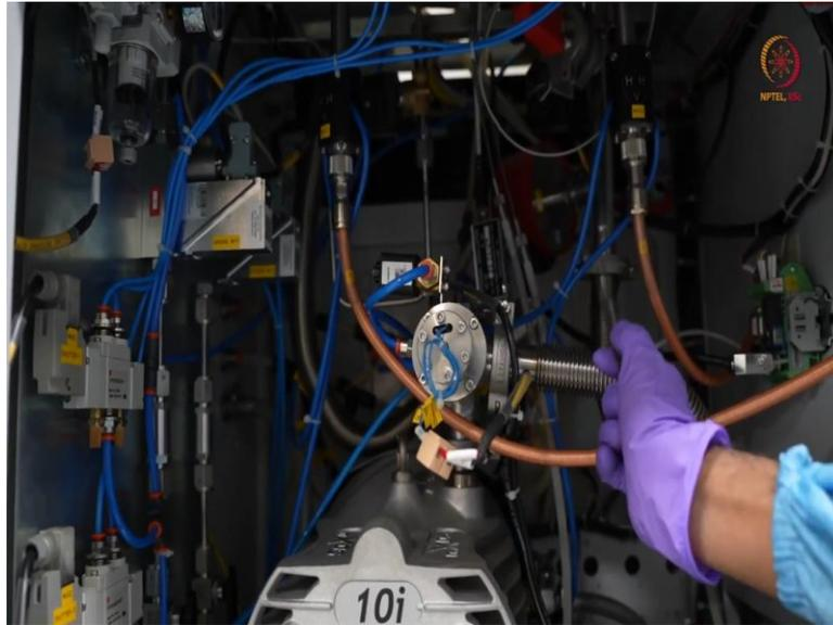
And if we can see through this area, so here as we have discussed about this, so here you can see the connections one from the side, another will be from that side, from backside basically, and both are with a tee it is connected here. So, one of these is the backing line, one of these is the roughing line. So, apart from this, we can see many things here.
