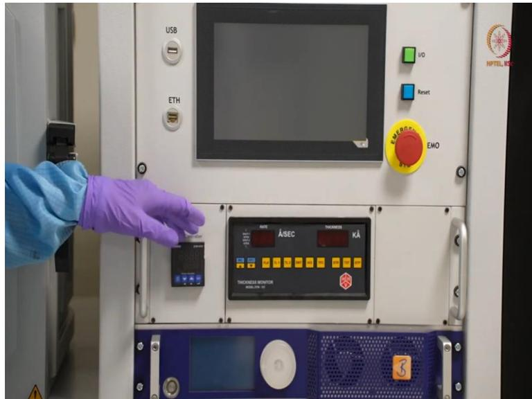
So, here, we can see here, this is the temperature controller. It is as it is written already. So, when we will operate the tool, we will show you. So, the top part that will show the actual temperature. And bottom here it can show what is the set temperature. So, with this we can elevate the temperature and at an elevated temperature we can deposit materials.
