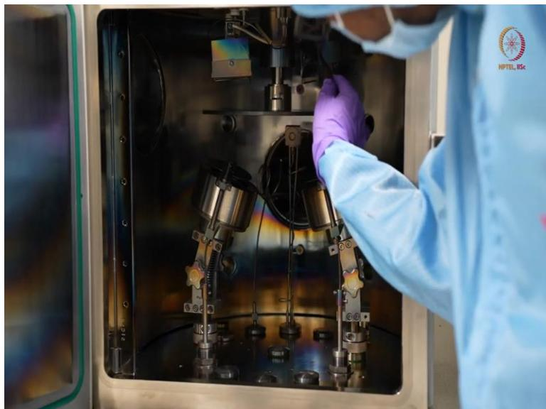
So, this is inside. Let us have a closer look, what is there in the chamber. So, this is inside the chamber as I have told already, that we have a provision for deposition at higher temperature. You can see here this and this here are the heaters. So these are the heaters that can directly heat our chuck. So the chuck is loaded here over the shaft. We will show how to remove and how to load the things. But still here are the heaters at the two ends.
