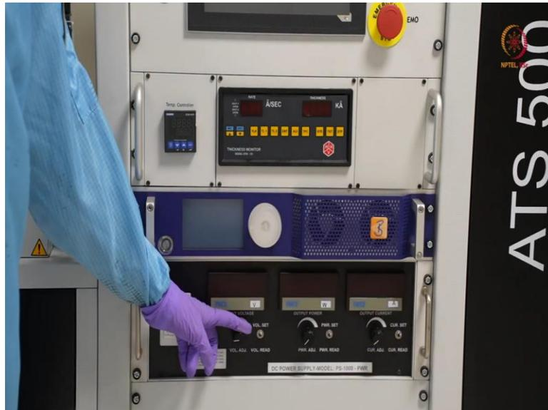
And here this is the DC power supply. So, if we see, we can just, it is always switched on. And here you can see three displays. So here are three displays, three buttons to increase or decrease the values. And here set and read, like set and read. This change for each and every parameter. Here first, what do you usually do is, in this DC source, this can support up to 800 volt and 1.5 ampere current.
