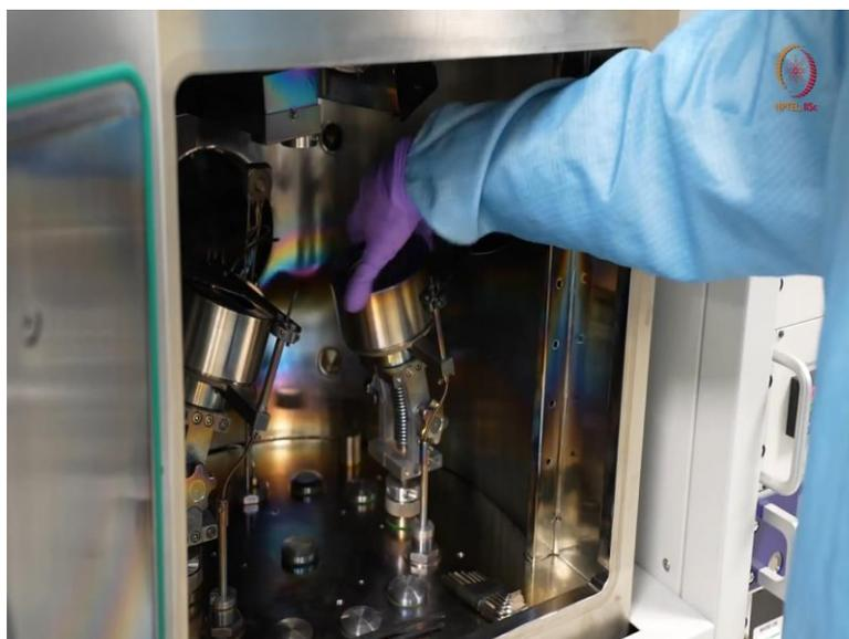
And now, this is the ground connection, this will just keep it, so you have to make sure that this part is clean, otherwise, this can be seen as a short connection. So before that, let us just press it. This is just like closing a container. And one thing just make sure after you load it, there should be a gap of 2 to 3 mm millimeter, 2 to 3 millimeter. So, this match gap and whatever voltage you will apply divided by this much gap.
