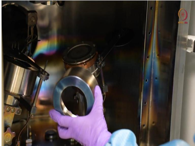
Here, you can see the closer look of on magnetron. So, how we are giving the instructions through the tab or through the display, interactive display that will show during deposition, but for now, we want to show what is there inside. So, first we are just removing the shutter. So, you can see, we can remove the shutter that is also pneumatic.
