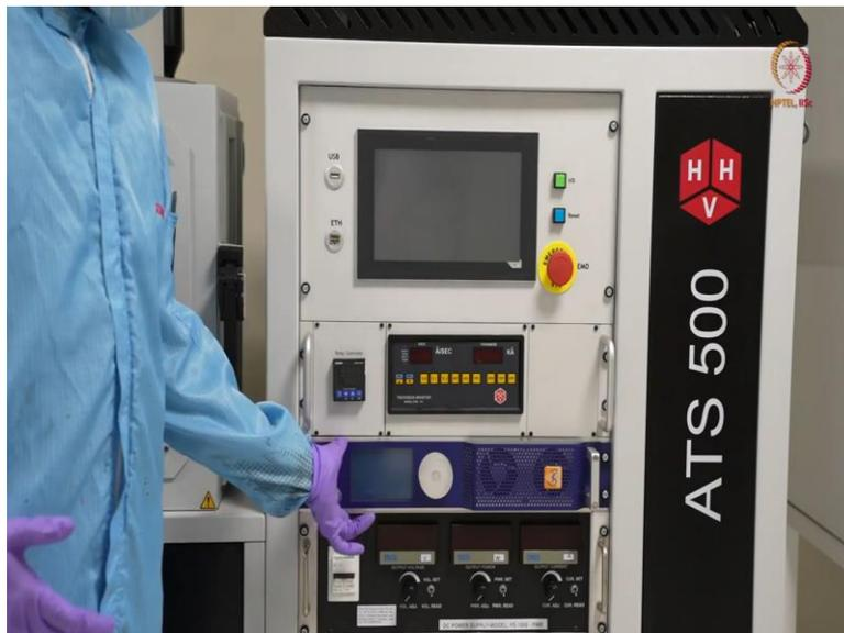
So here, this is basically the RF source. So as I already mentioned, so just to give a brief about this tool, we have two magnetrons, one magnetron is connected to the RF source and another magnetron is connected to the DC source. So here this is the RF source. So we can control this from this display only. So, we will just set the power and the forward power, reverse power, everything will be automatically taken care of by this module, this is the power source, power supply.
