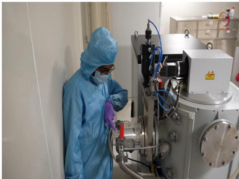
So, after those ports, now, we are at the backside of the chamber. So, here we can see this is the turbomolecular pump. So, this turbomolecular pump here you can see, one inlet water and outlet water. So, this also requires some chilling, some chilled water to get, I mean use it as a coolant. So, here is the turbomolecular pump, you can see, it is attached here like this with o-rings and all other connections.
