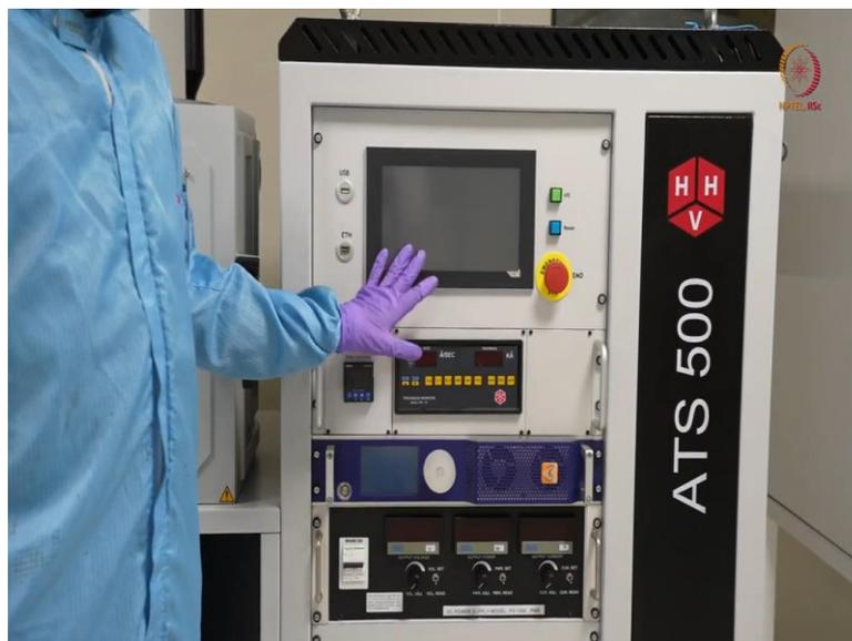
So, coming to this part. Here, first this is the display. So, whatever operations we are doing, like let us say creating vacuum, let us say triggering plasma, gas flow, switching on gas flow, switching off gas flow, heating, all these things, whatever we can do, we have to do it, I mean, we can give the instruction through this, this is a touch panel based. Here, this is that like one zero button like that, it was in EBM evaporator tools also.
