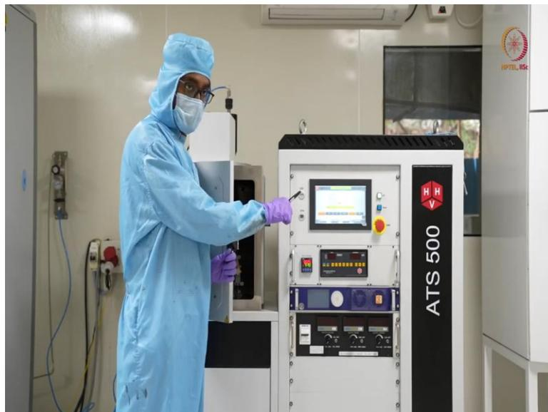
So, as I pressed vent, so vent is in green color that you have seen there only when it was a closed view. And it was showing an admit valve open. So it will be open until and unless we have enough air inside to open the chamber. That means releasing that vacuum and take this to the atmospheric pressure, then only we will be able to open the door. So we will wait till that time, we are waiting now also.
