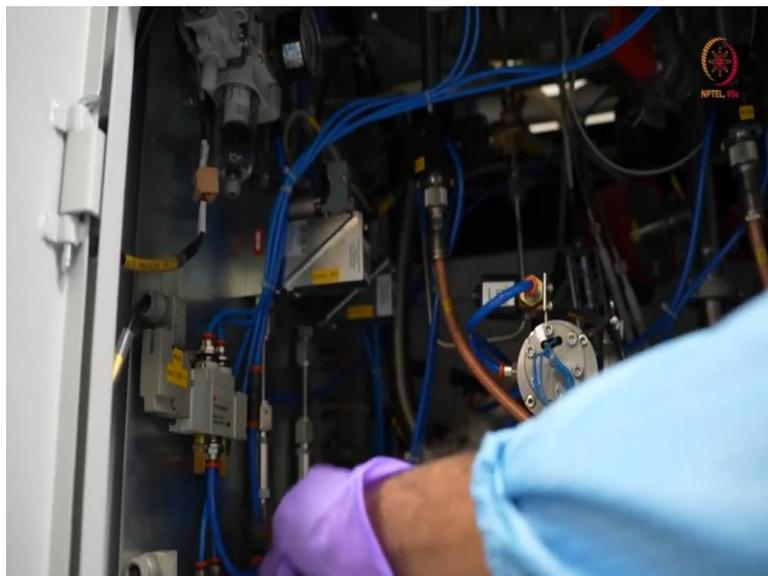
So, see here, this is the magnetron one for sputter one. So, this is one of the supplies. And here this is magnetron two, for the sputter two, this is another supply. These are the supplies for the water, whether water is going properly or not these are the cooling waters here, okay. This is the first thing.
