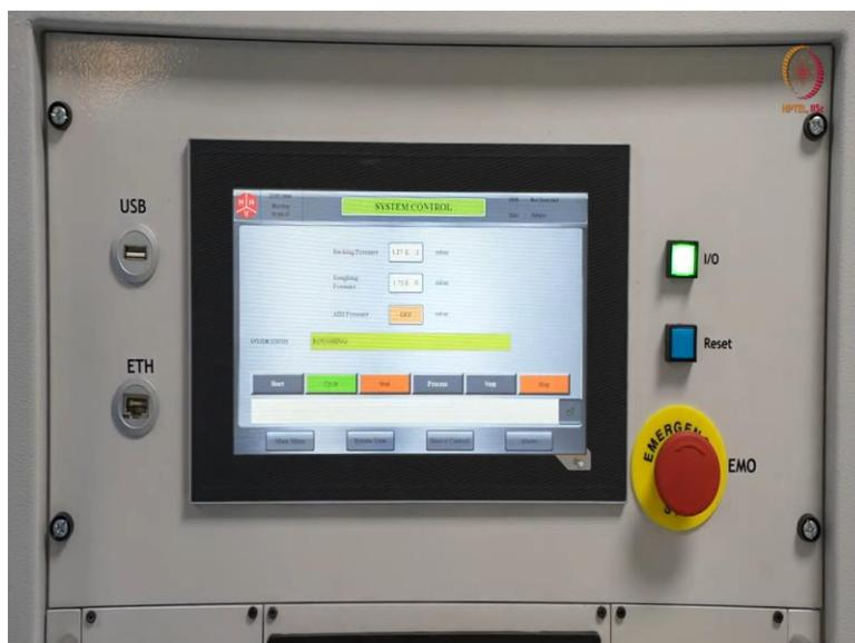
Let us go back to system control here, so that after roughing we will see, till high vacuum valve is ON or it will start high vacuum like cycle. After that we will take a like, in offline, we just create the vacuum then we will come back for deposition again. But till the time just wait, hardly It will take few more minutes from roughing to back into this.
