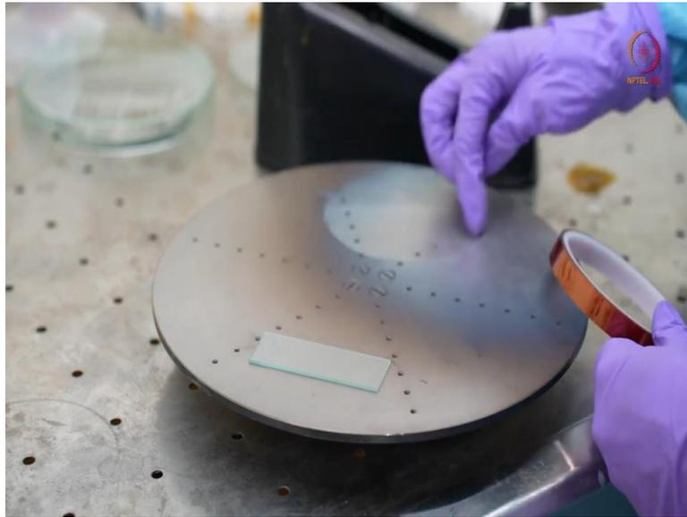
So, here you can see impression of one 4-inch of work. earlier we deposited, so that impression is still here. And after one deposition or two depositions, you have to clean the chuck.
