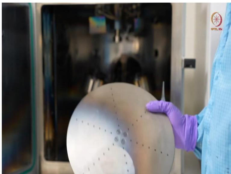
So here now, coming to this part. Here you can see the similar or before that I will just unload this so that you will get a clearer view. So this in the same way it can unload the chuck. So this is a little smaller chuck than that. This is eight-inch diameter. Whereas that I mean in case of EBM evaporation tool that we have that has 12 inch chuck, this is 8 inch only. That depends on your requirement, you procure it as you want.
