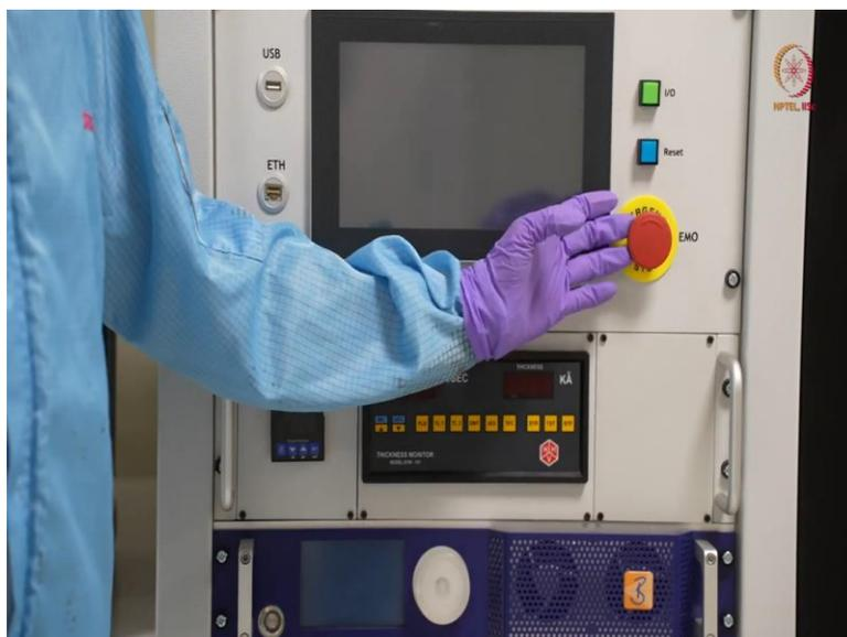
So, this is for switching ON the things and this reset button for resetting the hardware after each and every use. This is again one of the most important part. This is that emergency stop switch. So, if you are in any emergency or if something happens, you can just press it. It will like autocut the tool and you can just open it, before next use. There is nothing.
