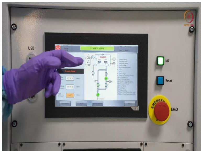
We can just get on better idea about this process from this system view. If you see this is the, I mean this is the chamber here, these are two magnetrons and here there are the connections like one MFC is dedicated to argon and the other MFC is dedicated to oxygen only, but you can use nitrogen as well, anything you can use here.
