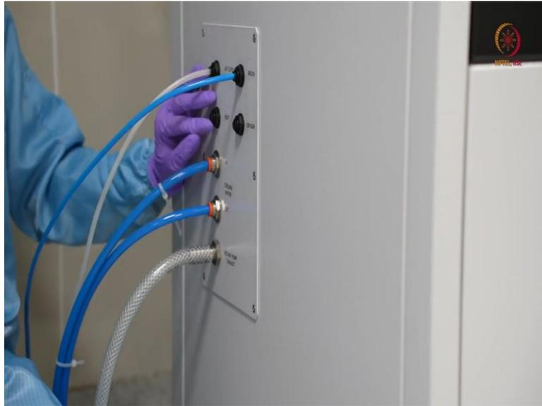
As you can see, we have closed the door. So, we are now here, the other side of the tool to show these things. So, here you can see, this is the air supply return. So, this is the pipe that is directly from the compressor. So, this compressor, I mean through the compressor will get some particular amount of basically you can say a rated pressure there. So that the rated pressure will be controlled by this compressor output.
