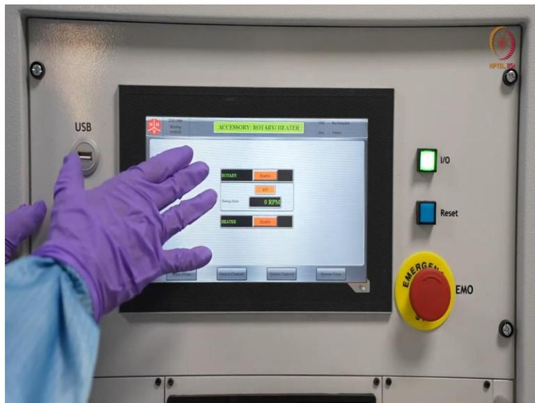
So, from here this is basically accessories. So, here you can check or you can start a rotation of the chuck or you can use heater. So, these are the basic features that we can get here.
