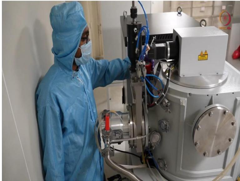
So, here you can see, I mean this is a penning gauge it works what we can show here, this is a penning gauge, Edwards, what can show here, this is a penning gauge that can show us the pressure less than  $10^{-3}$  millibar range to  $10^{-8,9}$  millibar range. So, we have it here. So, we have checked our chamber can reach up to  $10^{-1}$ ,  $10^{-6}$  millibar approximately. So, that makes this chamber can reach, that can be easily covered by this penning gauge.
