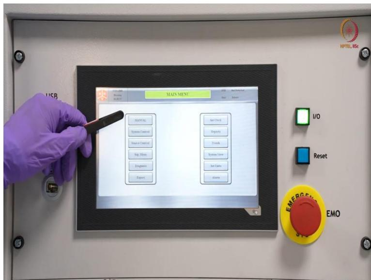
So, here if you see, anyway do not go with the date and time, this is not set properly. So, here if we see, this is a manual mode. So, if we want to run the tool in manual mode, we can go with that. But this is semi automated tool, where only deposition is manual, other things can be, can run automatically. So, here even deposition can be automated.
