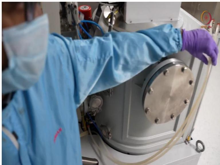
Here, if we come to this top part, so here, inside we have the rotary drive. So that rotary drive is to rotate the chuck during deposition. And here we have another port that we can open just like this we have another port. So here, we can use some load lock system, so that our chamber will be always under high vacuum and we can just load our sample here.
