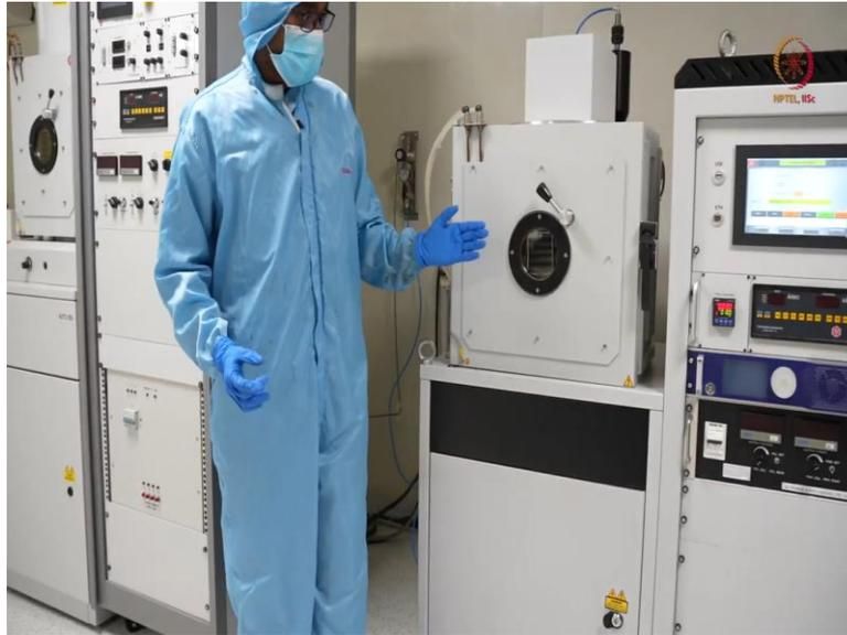
And through here. So, as we know air admit valve is here. So, through this venting is happening. So, air is going in, we will just open the chamber and see what is actually, how much was the deposition.
