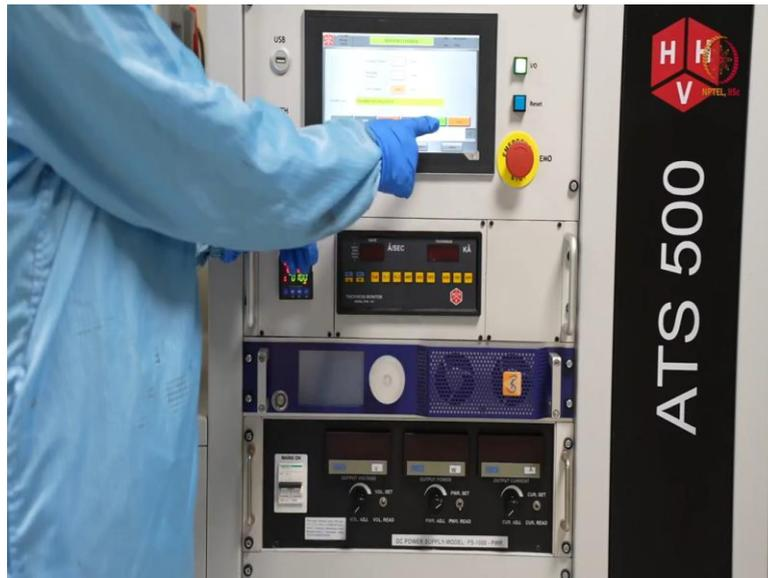
So, as I pressed vent, so, it is showing chamber vent sequence and then air admit valve open.
