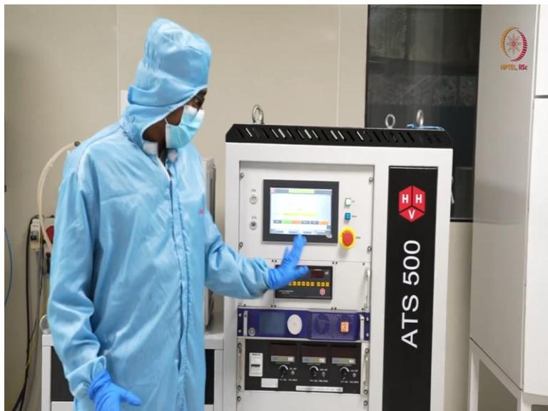
And another thing is we are about to off the tool. So we know that we are not going for further deposition. So, mandatorily, we have to switch off the gas supply. So, that we will do first. So, by the time it is creating some vacuum, by the time our gas flow is off already, though valve was off. So, gas flow was not there inside the chamber, but still it is better to be off.
