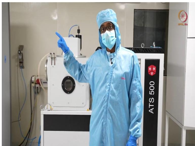
So, after this we can switch off the tool. So just press this. So, after this tool is shut down from this part, still we have to switch off the main power first, then chiller and compressor, these two have to switch off. So that should be in our mind, okay.
