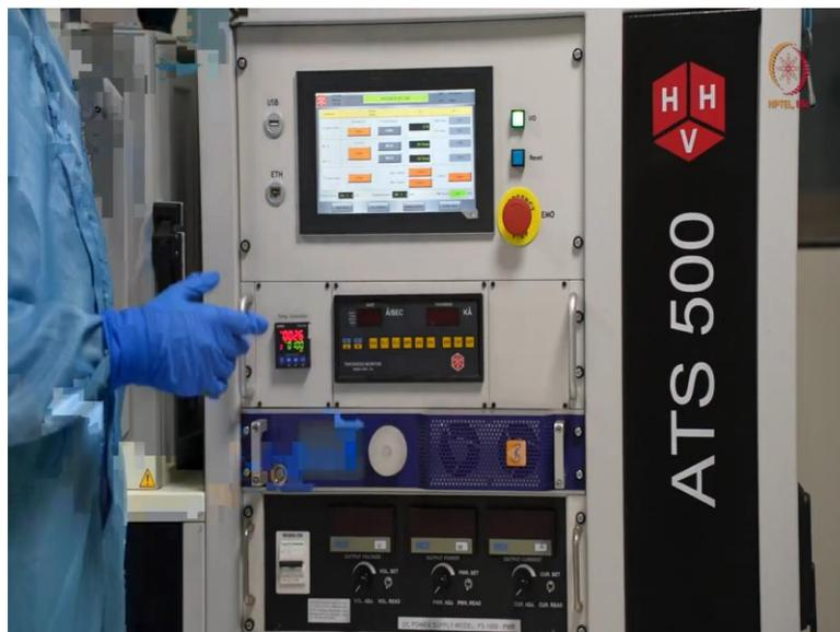
So coming to the next part, we will go to source control now. So here, here it will be like all the menus available. So here if you can see here, like the first one, we have provision for RF power as well as DC power. And we have provision for MFC like Mass Flow Controller, argon, oxygen. So, whatever we can, we want to choose, we will choose in that way.
