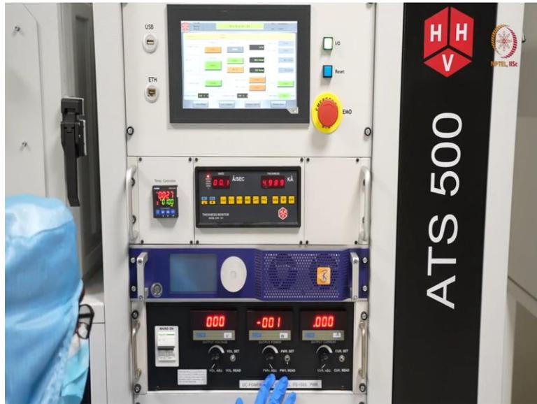
So, now decrease this voltage. So, this is zero, this is also zero. Here, you can keep this set or it is recommended to just minimize the power also and set it each and every time. Here after all this, you can actually switch off this DC power. It was enabled. So I just disabled it. So then this part is off.
