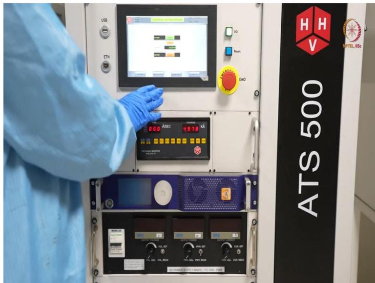
So, for that, we just came to that ACC control again and we change this rotary drive to 10 rpm, it was set at 5 rpm. So now we just set it to 10 rpm. So, this will, I mean uniformity can be governed by this. So, you have to change this 5 rpm, 10 rpm everything that you can, actually, you can like optimize the parameters as per your tool.
