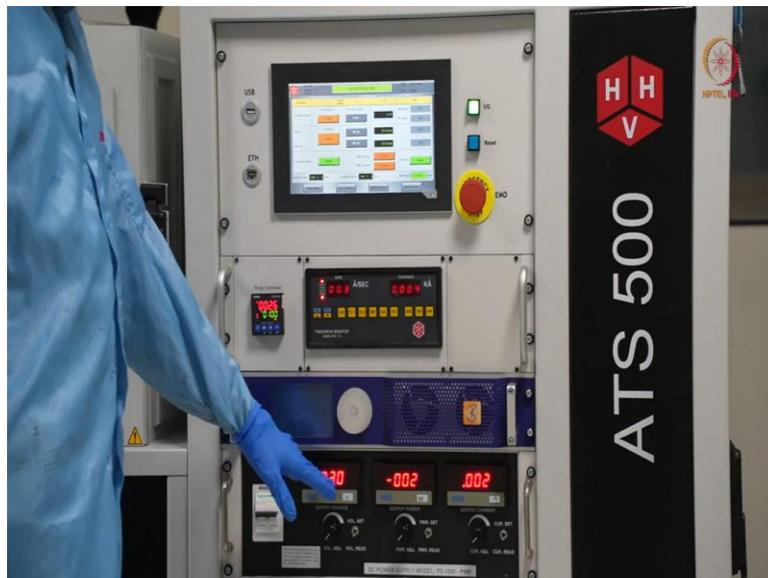
So here we have both options RF and DC, we will enable the DC supply. So just after enabling, you can see that here, this was on. So now you can see here, it will I mean, we will change it in such a way, so that plasma will be generated, we will go to that step. But before that. So, here we will switch on the MFC and for argon.
