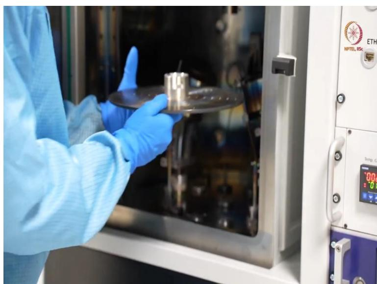
So, here we will, so, whenever we leave the tool, it is actually kind of mandatory that you close the chamber always. So, that will help you to manage with minimum contamination level of the chamber. So, we will just keep it in as we have already shown how to place it back or take it out side. We are not again showing the things. So, now, this is already inside.
