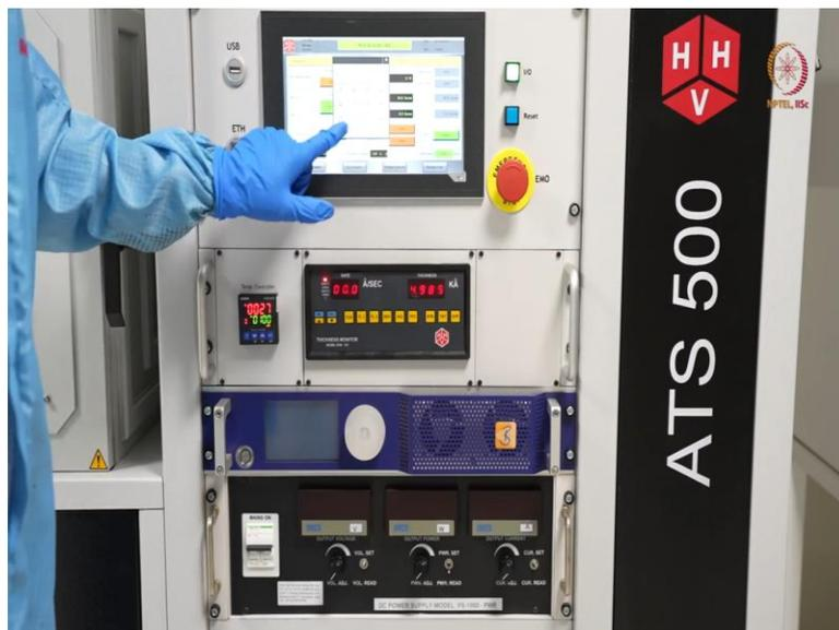
So here, gas flow actually, we can just reduce it a little bit or we will just reduce it to 20 where it was. So, after that, we can switch off this argon supply also, disable and disable. So, this will switch off that MFC part. So, this is something like everything comes under one deposition of DC sputtering. So, after this on the same sample, we will show you the RF sputtering as well.
