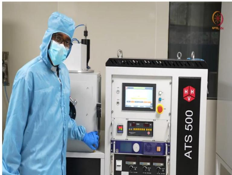
So, as you have closed the chamber, actually, we cannot leave the tool like this, because this is a vacuum tool that has a vacuum chamber here. So, if you leave the vacuum chamber at atmospheric pressure or under atmospheric pressure, so, actually efficiency of the tool will be lost or it will be compromised in long term. So, always we should keep it under vacuum.
