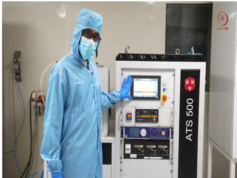
So, as you can see here, we left it for quite a long time and it is already minus 5 range. So, you can see here it is almost, e to the power minus 7.5 or e to the power minus 5, and it is still decreasing. So at this stage we can actually switch it off or turn off the tool. So, we have to wait till this much, otherwise, enough vacuum will not be here.
