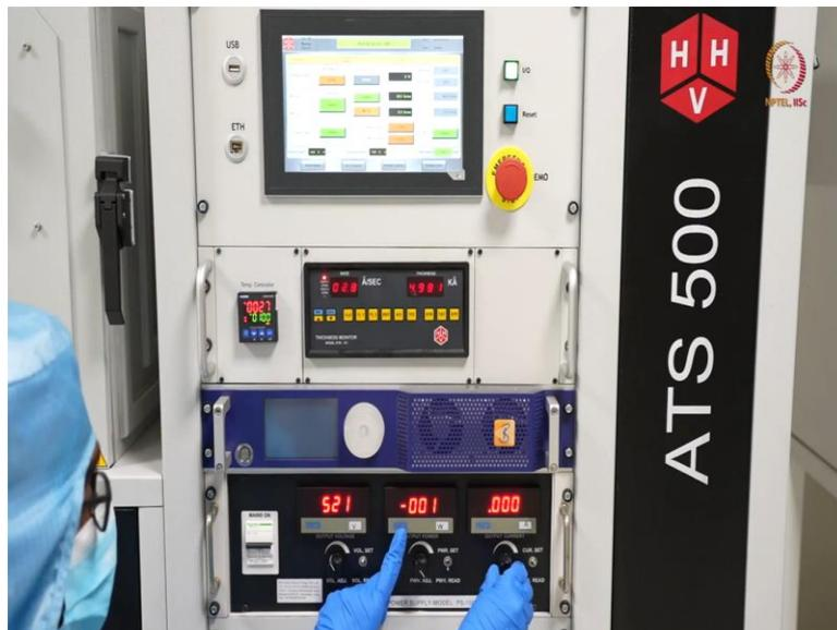
So, for that the first thing you have to do is close the shutter. So, just like same as electron beam evaporation technique, first close the shutter. So, the deposition will be stopped, after that decrease the current. So, with decrease in current, you can see that here output power will keep on decreasing. So, if current supply is has currently stopped, this is also zero.
