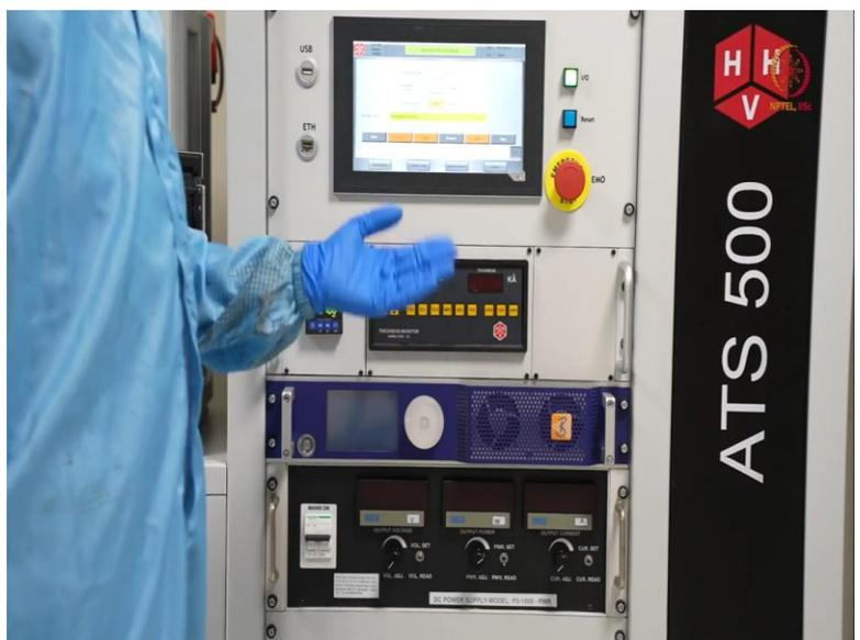
This step is almost similar, whatever you have seen in case of electron beam evaporation. So, both are from like similar make. So, options are also kind of similar. When a chamber is sealed, so, we have to go for venting to open the chamber.
