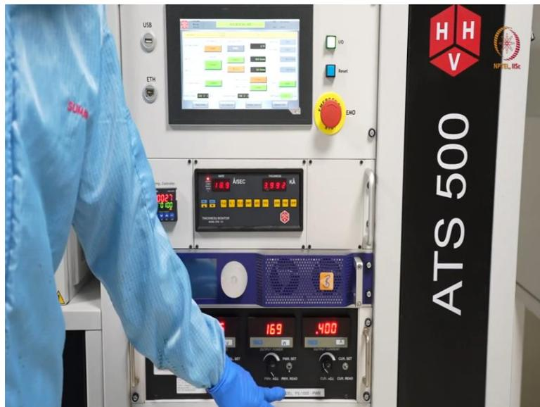
So, here as we mentioned, I change this to identify now. So, when you, I mean when we first focus inside, it was 400, now it is 525. Second, this one, these also have increased. So, that that effective power, I mean power delivered. So, we can we put it to power read. So, this is actual power delivered, this also increased to 170 and that is why that was the like, that was the plasma colour and that much of glow intensity that you saw there.
