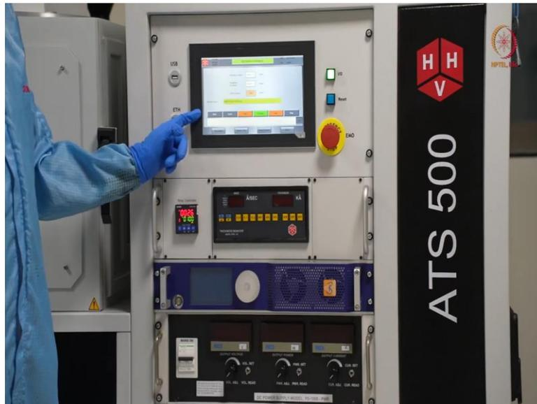
So here after the argon, we are pressing here process. So, in process mode, first throttle pumping will start. So in that way, I mean the pump down step or the suction by the vacuum pumps, it will not be in full, it will be like almost like half open type or the partially open type.
