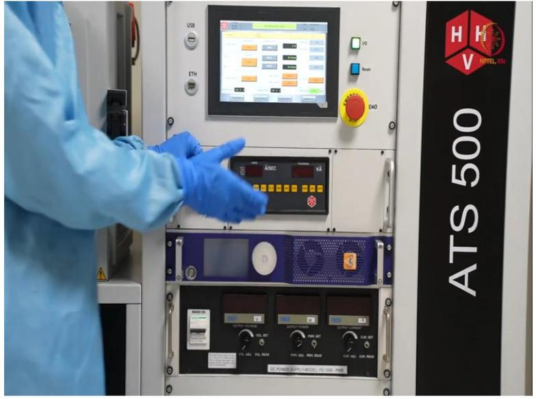
So, as you can see that we set it at zero watt. So, now it is zero. Now we can switch it up. So this part is done. Now here, if we consider this mass flow controller, this also have to switch it off. So first zero. So, flow will be stopped. Then disable that MFC argon and then close the gas valve. So this part is done.
