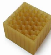
Honeycomb structure made using PEI material
