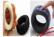
Tires printed using TPU material
