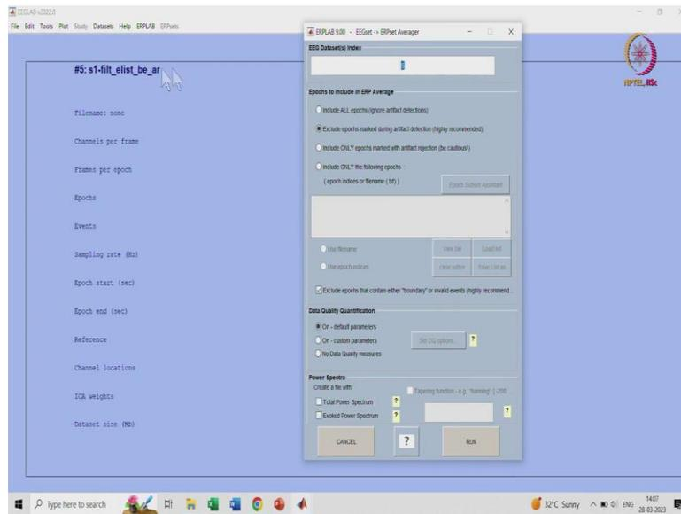
Last step is to generate a computed average ERPs so that will be saved as a final this you can select which data set you want to average here again what are your parameters and all you have to exclude epoch's Mark during artifact rejection. So, this is important you should not include all the epochs because you have identified that which particular epochs having non neural High amplitude so that you can remove and again you run it.
