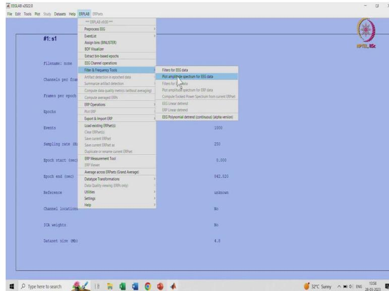
So there what you can do is you have to see that what is the current frequency spectrum that you can use a plot amplitude Spectrum from the ERP lab function. Again, ERP lab is a plug-in which should be added into the path in EEG lab which I already added how to install ERP lab as I mentioned I will put a link of my previous video in the description or comment you can go through that.
