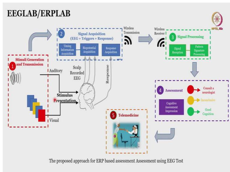
Provide you the recap this is what we have already learned in one of the course that will generate a stimuli followed by signal acquisition which will be wirelessly transmitted to a computation system and where you process and make the sense out of it. Assess something and it based on based on the application your final assessment varies.
