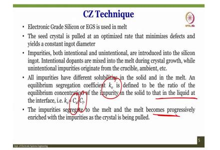
So, CZ technique is electronic grade for use for electronic grade silicon and the seed crystal is pulled at an optimized rate. So, like I said here like you are let us understand it a little bit slowly. So, the seed crystal is placed here once this molten region is there and then it is pulled. Pulled in this direction like this from the hot let us say this is hot to the cold side it is pulled when it is pulled it is also rotated like this.
