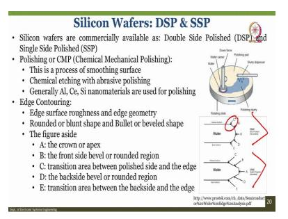
Now, we talk about this DSP and SSP as I told you earlier, either you have single side polished wafer or you have double side polished wafer and the way to polish the wafers is using the polishing mechanism either it is chemical mechanical polishing, or it is just a mechanical polishing. So, this process is used for smoothing of the wafer surface, we know that the smoothing is such that the wafer surface is almost few nanometers in the roughness.
