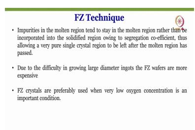
So, the impurities in the molten region thus tend to stay in the molten region rather than be incorporated into the solidified region owing to the segregation co-efficients thus allowing a very pure single crystals to be left after the molten region has passed.
