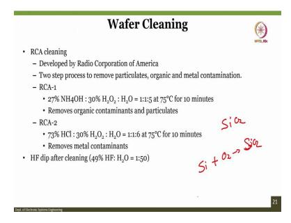
Now, once you have wafer even it is a new wafer, there is a formation of thin silicon dioxide. Why because silicon when reacts with oxygen forms sio2. So, if the oxygen present in the air will also cause a thin layer of silicon dioxide to avoid any kind of oxide when you start the wafer processing, it is important that you clean the wafer that there is something called RCA cleaning RCA-1 and RCA-2 the first RCA-1.
