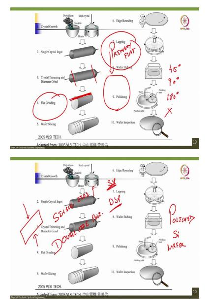
Now, let us see the FZ technique video so you have seen the video of the FZ technique as well. Now, let us understand the ingot, whether it is through CZ or through FZ, how we can create the wafer from the single crystal ingot, that is very important to create a wafer.
