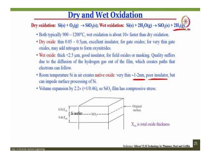
So, in this case you can see dry oxidation and wet oxidation the dry oxidation is silicon is which is solid when it reacts with oxygen which is not gas form it forms silicon dioxide and for the wet oxidation it is  $SiO_2$  plus  $H_2O$  gives  $SiO_2$  plus  $H_2O$  gives  $SiO_2$  plus  $H_2$  balancing equation  $2H_2$  balance equation here  $2H_2O$ .
