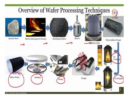
So, there are two different techniques one is called CZ technique also Czochralski technique second is called float zone technique (FZ) float zone technique and Czochralski technique. So, you start from the quad side rock and then you have electric submerged arc furnace, you can get
