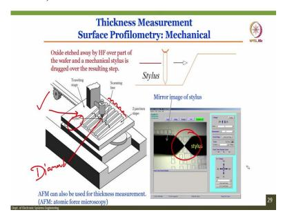
In this case, which is a mechanical way now mechanical way the disadvantage of this limitation of this is that we need to create a step. When you create a step that means that you are destroying that particular material, what does it mean?
