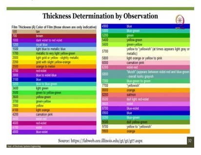
So, in reality it is this complicated. So, you see that right from 10 all the way to blue violet how the thickness changes and how the colored bands are there. Same thing goes for blue all the way to 9900 thing which is orange. So, generally when you see the silicon oxide or oxidized silicon wafer, you will see either one of these particular light.
