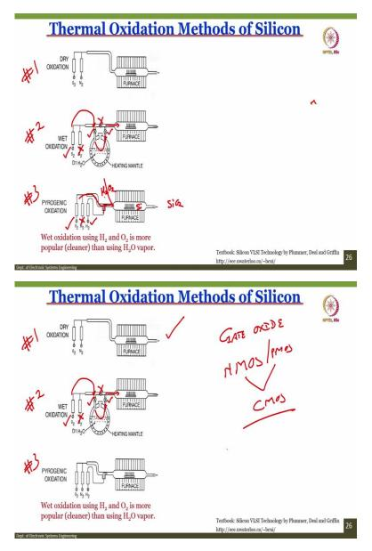
The last one, how it works? There is a pyrogenic oxidation, pyrogenic oxidation does not require you to have a bubbler and water vapour. But instead of that what happens is initially only nitrogen is open, hydrogen is closed, oxygen is closed, nitrogen will flow through this all the way here into the furnace and the wafers are placed in the furnace in presence of nitrogen.
