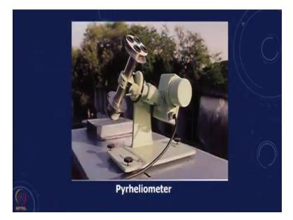
We are looking at the direct and diffuse, so we have a direct and diffuse, if you looking at direct isolation, this is an instrument which is used to measure the direct beam insolation, this is called the Pyrheliometer, this is focus, so that it is directly depending on the position of the sun, it will be taking the direct normal beam radiation to the sun and you have this is measurement.
