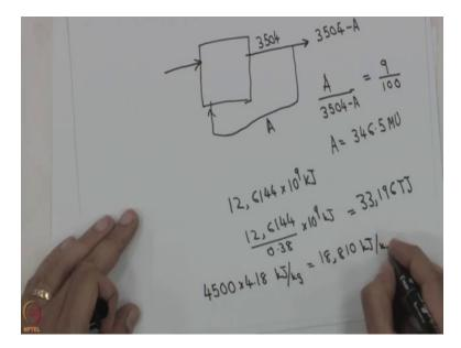
Now, let us look at this was the gross generation, we were talking in terms of the auxiliary consumption. So, if we look at a power plant we have an input and we have gross generation this gross generation is 3504 MUs out of which we have an auxiliary consumption 'A' being used and this net which we get is 3504 minus 'A'. So, let us calculate, we are told that 9% is the auxiliary consumption, which means
