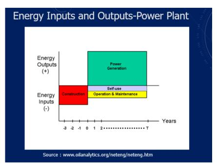
If you look at a coal-based power plant. There would be the energy inputs are all provided in the initial year. When it is start operating there is whole set of embodied energy because you have the steels, you have all the material which are coming in to the construct the power plant.
