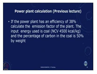
So, let us just recast that question – If this thermal power plant has an efficiency of 38 % calculate the emission factor of the plant. So the input energy used is coal with net calorific value of 4500 kcal/kg and the percentage of carbon in the coal is 50 % by weight.
