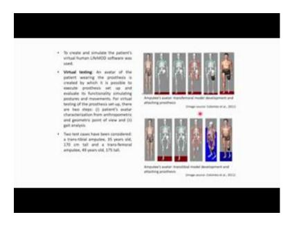
So, this is that middle portion. In the middle portion, all these information's are collected. Then, socket design creates 3D virtual model of the socket around the stump digital model acquired with the reverse engineering equipment. This step foresee socket modeling assistant and finite element analysis tool to study the stump socket interaction
