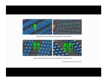
From this image it is visible that while the chairs are arranged in block form. So in between 2 doors of chair the space is sufficient so that one 95th percentile or people with larger body dimension can easily go inside and come out. So here you can see the chair arrangement. And in between 2 blocks of seats or chairs the space is sufficient for movement of at least 2 people side by side with larger body dimension. So that is also shown here.
