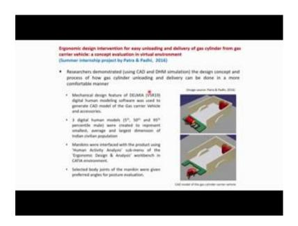
The next project it was by Patra and Padhi in 2016, in this summer project they carried out research on ergonomic design intervention for easy unloading and delivery of gas cylinder from gas carrier vehicle. So researchers demonstrated using CAD and digital human model simulation. The design concept and processes of how gas cylinder unloading and delivery can be done in a more comfortable manner.
