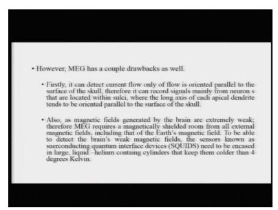
Now MEG, although it is very advantageous, as I said, it has a couple of drawbacks as well. Two very important drawbacks are that basically it can detect current flow only if the flow is oriented parallel to the surface of the skull. So that kind of eliminates a lot of regions, which will generate a current not parallel to the skull.
