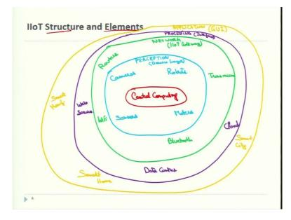
So, there is a structure and elements of it. When I say structure, there are layers of the Industrial Internet of Things. If I tried to name those layers, they are perception, network, processing and application. So, I have first at the center of central computing.
