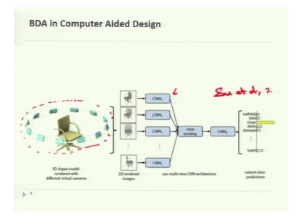
This figure is taken from them, where a chair 3D shaped was to be made, circular vise the camera take different pictures of the chair, we can decide number of pictures to be taken, which are fed as an input to the CNN here, to different neural connections that are there, a 3D shape can be recognized even from a single view at an accuracy far higher than using a state of our 3D shape descriptors or so.
