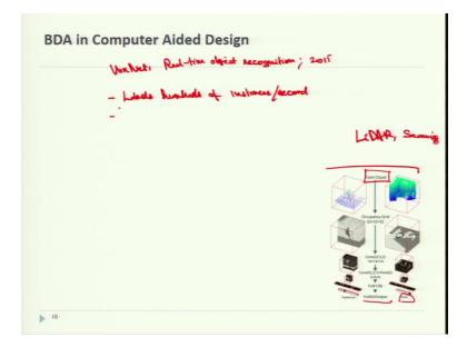
Another study, in which Vox Net architecture, Vox Net architecture are given. This is a Vox Net architecture in which you have a plant cloud data and the occupancy grid and we have a convolution layers and finally, we try to have a full output layer which helps us to let us know that whether the shape that was input here from the point cloud from the input data, which is the class it is falling in, where it is showing it falls in that class of twilight, maybe.
