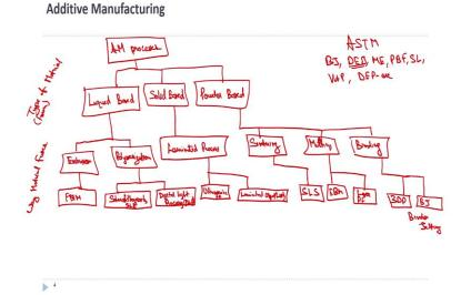
Let us now talk about the general things about Additive Manufacturing. Additive Manufacturing means when we keep on adding the material layer by layer. The difference from subtractive manufacturing is that other CNC machines generally reduce or remove the material. Additive Manufacturing keeps on adding the material and the material is being, when being added it has to be added layer by layer, the different methodologies or different material types that we use in Additive Manufacturing.
