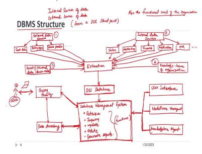
Now let us get into DBMS structure and we will try to study this in a schematic form. So, remember we have talked about internal sources of data and external sources of data earlier. And we also talked about the private data etc. So, database structure from a DSS standpoint, we are going to do is, we are going to look at from a DSS viewpoint.
