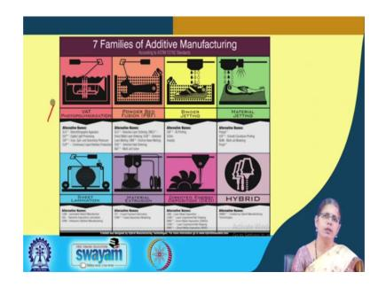
So, this illustration represents the standard way of looking at the area of additive manufacturing, there are 7 different ways in which additive manufacturing can happen. The first one is what we call vat polymerization. This has certain way in which the technology is implemented.
