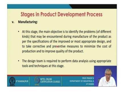
Fifth stage is manufacturing, At this stage, the main objective is to identify the problems (of different kinds) that may be encountered during manufacture of the product as per the specifications of the improved or most appropriate design, and to take corrective and preventive measures to minimize the cost of production and to improve quality of the product. The design team is required to perform data analysis using appropriate tools and techniques at this stage.
