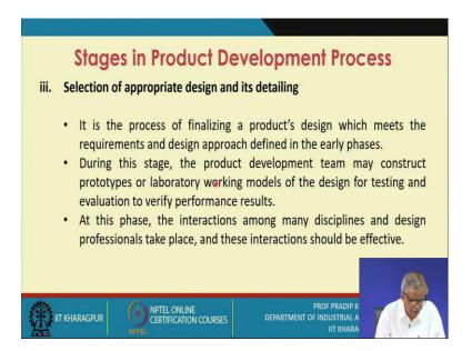
Third stage is selection of appropriate design and its detailing. It is the process of finalizing a product's design which meets the requirements and design approach defined in the early phases.
