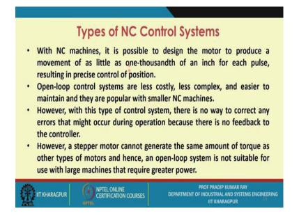
With the NC machines, it is possible to design the motor to produce a movement of as little as one-thousands of an inch. Open-loop control systems are less costly, less complex, simple and easier to maintain then they are popular with the smaller NC machines.
