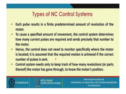
Each pulse results in a finite predetermined amount of revolution of the motor. To cause a specified amount of movement, the control system determines how many current pulses are required and sends precisely that number to the motor.
