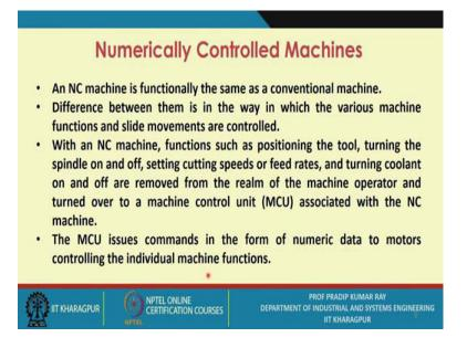
NC machine is functionally the same as a conventional machine. From the conventional machine suppose you are getting n number of functions or n number of operations, all these operations are needed or a necessity.
