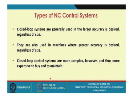
A closed-loop systems are generally used if the larger accuracy is desired. They are also used in machines, so greater accuracy is desired
