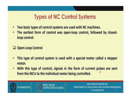
There are two types of NC control systems you come across. One is the open-loop control and the second one is the closed-loop control. Two basic types of control systems are used with NC machines The earliest form of control was open-loop control, followed by the closed-loop control.
