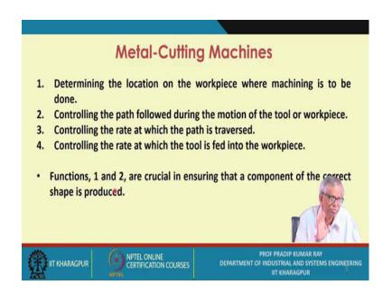
When you try to automate the system, automate the working of a machine tool, what kind of activities you are doing, what are the functions you should be aware of? First, determine the location on the workpiece where machining is to be done.
