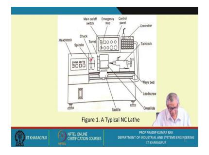
We are referring to a typical NC lathe. Head stocks, you have the spindle, the turret, the chuck and these are the switches, on and off switches, emergency stop, this is a control panel. The controller is the tailstock. You must be familiar with all these operations or a typical lathe.
