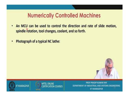
An MCU Machine Control Unit can be used to control the directions and the rate of slide motions, spindle rotation, tool changes, Coolant is to be used. Usually, the coolant is a source solution.
