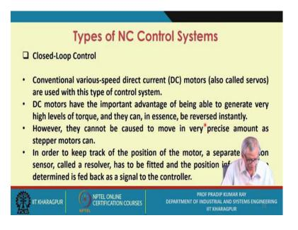
Alternatively, you can use the closed-loop control, the conventional various speed direct control, DC motors you have to use, also called the servos. These servos are used in this control system. Advantage is that a DC motor is able to generate very high levels of torque, and they can, in essence be reversed instantly.
