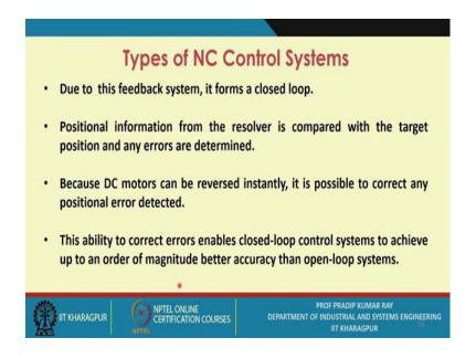
This is positional information we have to work it as the process is on, as the activities being carried out, the operations are being done. That is why the DC motors can be reversed instantly. The ability to correct errors enables closed-loop control systems to achieve up to an order of magnitude better accuracy than open-loop systems.
