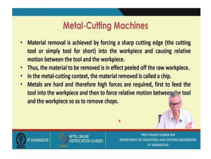
How do you get this the material removal process? You remove this excess material by forcing a sharp cutting edge. Here you have to force a sharp cutting edge that is the cutting tool or the simply tool into the workpiece
