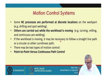
Now, let us talk about the NC motion control system. Because there has to be a tool path to be defined and the depending on type of operations you carry out, you need to define the motion control system.
