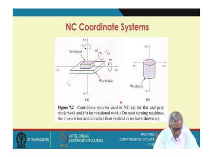
If you look at this particular figure, your understanding will be more perfect. When you use this three axes machine x, y and z, you find that there is work table on the machine tool and on the work table you place the work part in a particular location.
