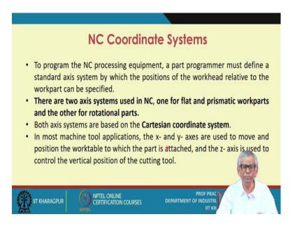
NC motion coordinate system is used for writing down the program for the part. So, you should have prior knowledge about the NC coordinate systems. To program the NC processing equipment, a part programmer must define a standard axis system. Cartesian coordinate systems, standard axis system by which the positions of the work-head relative to the work part can be specified. As soon as you try to define the positions or the location, certain coordinate systems you have to use.
