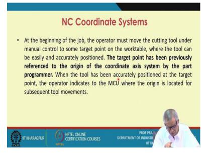
At the beginning of the job the operator must move the cutting tool under manual control to some target point on the work table where the tool can be easily and accurately positioned, means at the corner point, the table is located and you marked the zero point over there.
