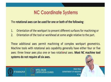
Normally this coordinate system altogether you have the six axis, x, y, z and a, b, c. Now why all these six axes required? Because NC machine tool is suitable for producing very intricate shapes and sizes. The entire process sometimes referred to as contouring.
