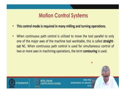
This control mode is required in many milling and turning operations.
