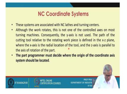
These systems are associated with NC lathes and turning centers. Although the work rotates, this is not one of the controlled axes on most turning machines, consequently the y axis is not used. So, only the x axis and the z axis you require for the rotational part.
