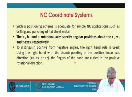
Such a positioning scheme is adequate for simple NC applications. like drilling and punching of flat sheet metal, sheet metal work is a very common in the work. When you go to the fabrication shop, there will be a sheet metal work of various types.
