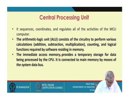
CPU coordinates is basically the brain of the computer. It sequences, coordinates, and regulates all of the activities of the MCU computer. Arithmetic logic unit consist of the circuitry to perform various calculations like addition, subtraction, multiplication, counting and logical functions required by software are residing in memory.
