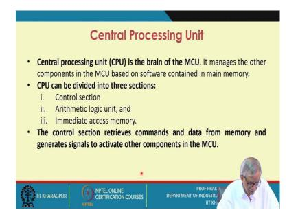
The CPU is the brain of the MCU that is known to you, it manages the other components in the MCU based on software content in main memory. CPU can be divided into 3 sections control section, arithmetic logic unit (ALU), and immediate access memory. The control section retrieves commands and data from memory and generate signals to activate other components in the MCU.
