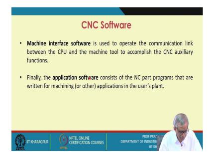
Machine interface software is used to operate the communication link between the CPU and the machine tool to accomplish the CNC auxiliary functions. With one particular CNC or in a particular CNC system; not only you can engage one machine tool, but n number of machine tools, a large number of machine tools.
