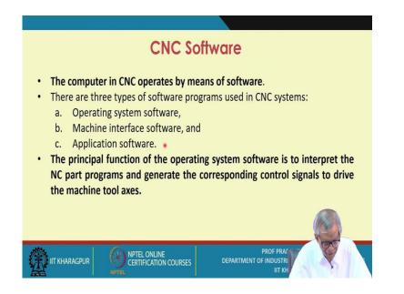
Now, you need to use several kinds of the software, let us have some the knowledge on this software what actually it does and why it is used. The computer in CNC operates by means of software. There are three types of software programs used in CNC system; three types.
