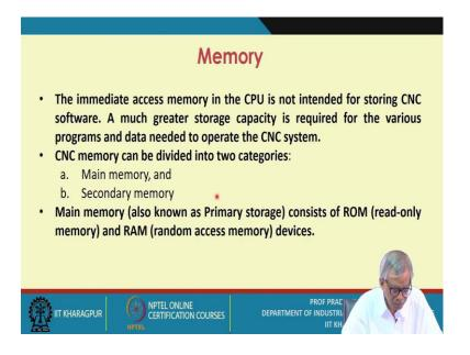
The immediate access memory in the CPU is not intended for storing CNC software. A much greater storage capacity is required for the various programs and data needed to operate the CNC system.
