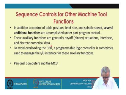
The next one is the sequence control. There is a process plan and there is a sequence of operations to be carried out. In addition to control of table position, feed rate, and spindle speed, several additional functions are accomplished under part program control.
