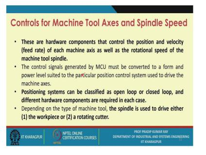
These are the hardware components that control the position and velocity for feed rate of each machine axis as well as the rotational speed of the machine tool spindle. These are the two important aspects we referring to.
