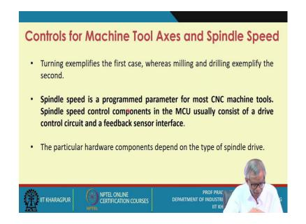
Turning exemplifies the first case, whereas milling and drilling exemplify the second one.
