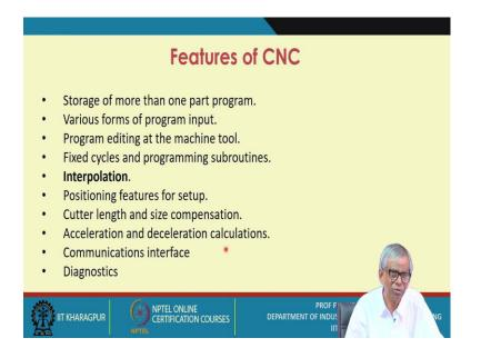
These are the features of CNC; the first one is the storage of more than one part program. Simultaneously you can store not only one part program, but you can store a large number of part programs.
