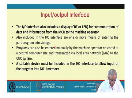
The I/O interface also includes a display (CRT or LED) for communication of data and information from the MCU to the machine operator. Also included in the I/O interface are one or more means of entering the part program into storage. Programs can also be entered manually by the machine operator or stored at a central computer site and transmitted via local area network (LAN) to the CNC system. A suitable device must be included in the I/O interface to allow input of the program into MCU memory.
