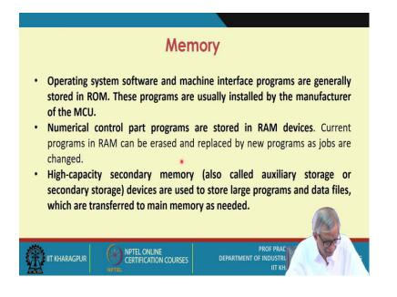
Operating system software and machine interface programs are generally stored in ROM. These programs are usually installed by the manufacturer of the MCU. Numerical control part programs are stored in RAM devices. Current programs in RAM can be erased and replaced by new programs as jobs are changed. High-capacity secondary memory (also called auxiliary storage or secondary storage) devices are used to store large programs and data files, which are transferred to main memory as needed.
