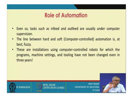
When you refer to flexible automation, re-program ability is an important characteristic, that means, if you want to produce another part, you write down a different program.
