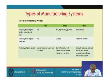
You just cannot start producing and altogether a different product in a continuous processing. Next important factor is flexibility to change to similar, but different part. Yes, for piece rate it is possible; if it is a batch production system, yes, if previously planned; that means, certain preparation is required and if you opt for mass production system, very limited.
