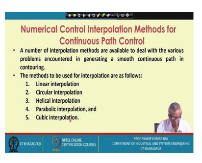
The number of interpolation methods are available to deal with the various problems encountered in generating a smooth continuous path in contouring. Basically, for contouring you have to use these interpretation methods. The number of the methods you can use define the continuous path or depending on the type of the continuous path. So, this continuous path could be linear, circular, helical, parabolic, cubic.
