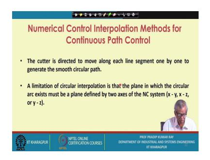
The cutter is directed to move along each line segment one by one to generate the smooth circular path. A limitation of circular interpolation is that the plane in which the circular arc exists must be a plane defined by two axes of the NC system (x - y, x - z, or y - z).
