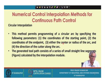
Next one is circular interpolation This method permits programming of a circular arc by specifying the following parameters: (1) the coordinates of the starting point, (2) the coordinates of the endpoint, (3) either the center or radius of the arc, and (4) the direction of the cutter along the arc. The generated tool path consists of a series of small straight line segments (see Figure 7.5) calculated by the interpolation module.
