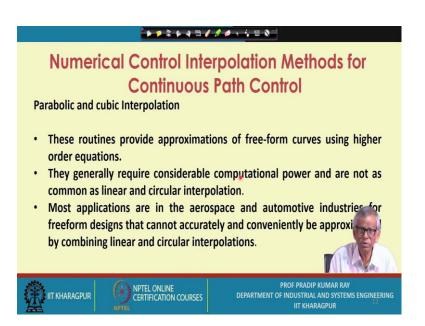
Next one is Parabolic and cubic Interpolation. These routines provide approximations of free-form curves using higher order equations. They generally require considerable computational power and are not as common as linear and circular interpolation. Most applications are in the aerospace and automotive industries for freeform designs that cannot accurately and conveniently be approximated by combining linear and circular interpolations.
