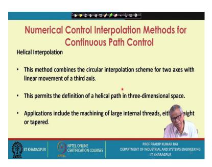
Next one is helical interpolation. This method combines the circular interpolation scheme for two axes with linear movement of a third axis. This permits the definition of a helical path in three-dimensional space. Applications include the machining of large internal threads, either straight or tapered.
