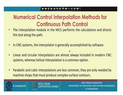
The interpolation module in the MCU machine control unit performs the calculations and directs the tool along the path. So, the tool path movement you have to do. In CNC systems the interpolation is generally accomplished by software. Linear and circular
