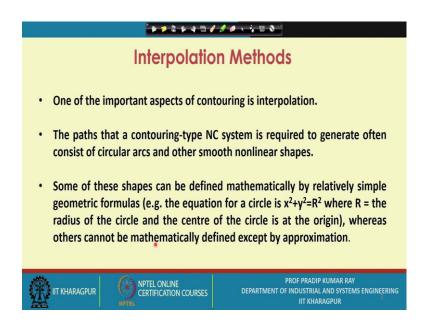
One of the important aspects of contouring is interpolation. The paths that a contouring-type NC system is required to generate often consist of circular arcs and other smooth nonlinear shapes. Some of these shapes can be defined mathematically by relatively simple geometric formulas (e.g. the equation for a circle is  $x^2+y^2=R^2$  where R = the radius of the circle and the center of the circle is at the origin., whereas others cannot be mathematically defined except by approximation.
