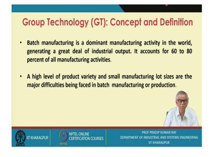
There are three kinds of the manufacturing system, first one is continuous processing and then job shop and the third category is the batch manufacturing or batch production and Batch manufacturing is a dominant manufacturing activity in the world, generating a great deal of industrial output. It accounts for 60 to 80 percent of all manufacturing activities. The
