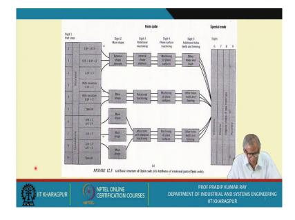
This is the basic structure. This part here, digit 1, digit 2, digit 3, digit 4, digit 5 and digit 6. The digit 5 now these are L/D, L/D means essentially if it is 0; L/D means dimensional envelope. This is basically for both of rotational parts, for the rotational part it will be L/D and for the non-rotational prismatic part it will be , length/width or they use a notation A, B. So, this is the first part.
