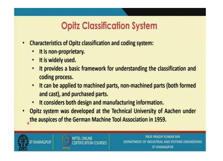
Opitz system has the following characteristics: It is non-proprietary. It is widely used. It provides a basic framework for understanding the classification and coding process. It can be applied to machined parts, non-machined parts (both formed and cast), and purchased parts. It considers both design and manufacturing information.
