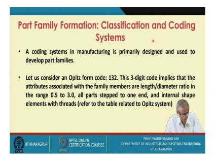
The basic objective is to part family formation. In the part family formation, these classification and coding system is to be used. A coding system in manufacturing is primarily designed and used to develop part families.
