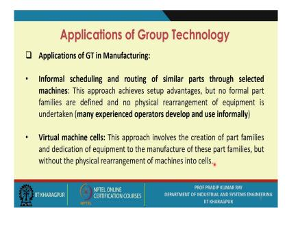
Group technology principles you can use in various ways. In a typical manufacturing system, you will find that operators will be on a particular machine tool may be producing or may be processing different type of parts in shapes and sizes, and over the years he is gaining experience.
