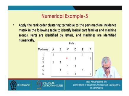
Apply the rank-order clustering technique to the part-machine incidence matrix in the following table to identify logical part families and machine groups. Parts are identified by letters, and machines are identified numerically.
