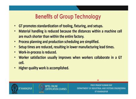
When you start using the GT principles, you will be going for simplification of the assembly design.
