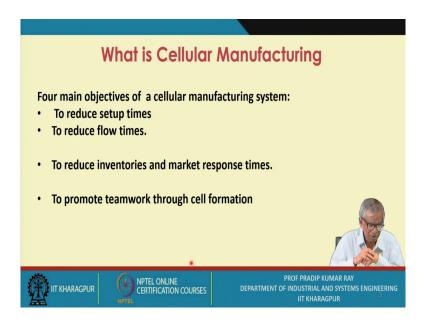
The four main objectives of a cellular manufacturing system, First one is the reduce setup times because individually all the machines have its own setup.
