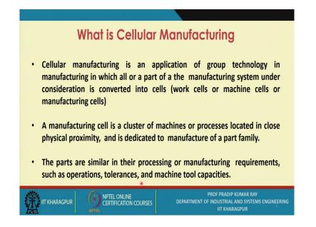
Cellular manufacturing is an application of group technology in manufacturing in which all part of the manufacturing system under consideration is converted into cells. The cells are normally referred to as the work cells or the machine cells or manufacturing cells.
