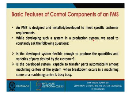
An FMS is designed and installed or developed to meet specific customer requirements. While developing such a system in a production system, we need to constantly ask the following questions.
