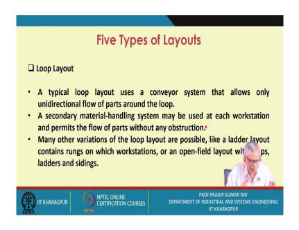
Now, the fifth one is the loop layout. A typical loop layout uses a conveyor system that allows only unidirectional flow of parts around the loop.
