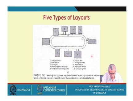
This is a typical example. This is your starting point, that is why it is 1. Then, it goes to over here; first one is the unload station, this is the loading station.
