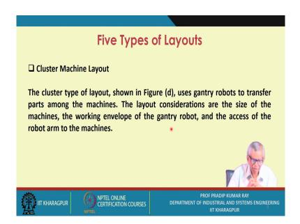
The next one is the cluster machine layout, where you can use different kinds of robots; the gantry robots are used quite frequently. The cluster type of layout shown in figure (8); the different types of the machines you have to use for the entire shop for the entire plant.
