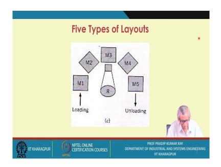
I will show you one particular figure. This is the robot. This is a robot envelope and this robot will be used for material handling, material transfer from one workstation to another.
