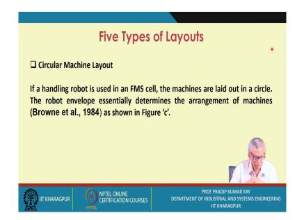
Second one is the circular machine layout. If a handling robot is used in an FMS cell, the machines are laid out in a circle. You must know the robot envelop. The robot envelope essentially determines the arrangement of machines.
