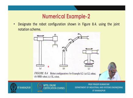
Second example; designate the robot configuration shown in figure. Let us talk about this particular robot configuration. This is linear, this is also linear movement taking place.
