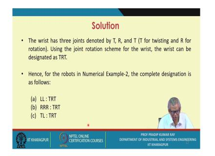
The wrist was having three joints denoted by T, R and T. T for twisting and R for rotation. Using the joint rotation notation scheme for the wrist, the wrist can be designated as TRT. Hence, for the robots in numerical example two the complete designation is as follows; LL:TRT RRR:TRT and TL:TRT.
