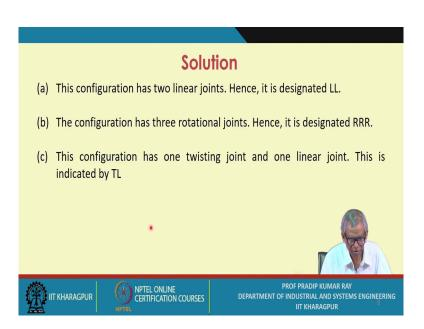
This configuration has two linear joints, the first one. Hence, it is designated as L-L. The second one is R-R-R.
