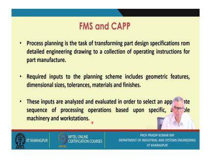
Process planning is the task of transforming part design specifications rom detailed engineering drawing to a collection of operating instructions for part manufacture. Required inputs to the planning scheme includes geometric features, dimensional sizes, tolerances, materials and finishes. These inputs are analyzed and evaluated in order to select an appropriate sequence of processing operations based upon specific, available machinery and workstations.
