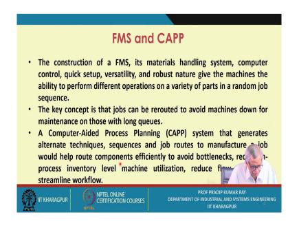
The construction of an FMS, the materials handling system could be the automated storage and retrieval system also is part of that. Computer control, quick setup. So, whenever we refer to quick setup sometimes, we refer to one particular Japanese technique, quick setup or accelerated setup.
