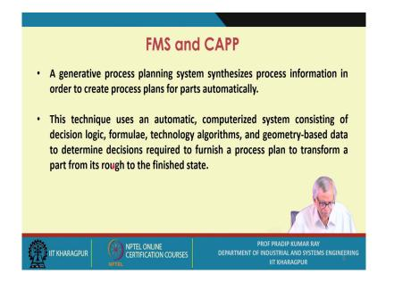
A generative process planning system synthesizes process information in order to create process plans for parts automatically. This technique uses an automatic, computerized system consisting of decision logic, formulae, technology algorithms, and geometry-based data to determine decisions required to furnish a process plan to transform a part from its rough to the finished state.
