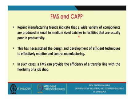
Recent manufacturing trends indicate that a wide variety of components are produced in small to medium sized batches in facilities that are usually poor in productivity. This has necessitated the design and development of efficient techniques to effectively monitor and control manufacturing. In such cases, a FMS can provide the efficiency of a transfer line with the flexibility of a job shop.
