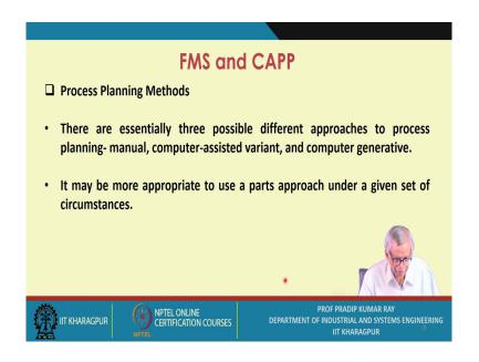
In the process planning methods There are essentially three possible different approaches to process planning- manual, computer-assisted variant, and computer generative. It may be more appropriate to use a parts approach under a given set of circumstances.
