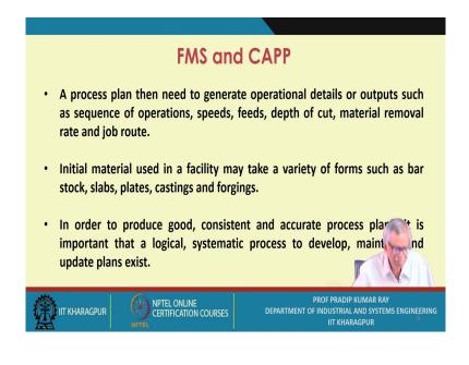
A process plan then need to generate operational details or outputs such as sequence of operations, speeds, feeds, depth of cut, material removal rate and job route. Initial material used in a facility may take a variety of forms such as bar stock, slabs, plates, castings and forgings. In order to produce good, consistent and accurate process plans, it is important that a logical, systematic process to develop, maintain and update plans exist.
