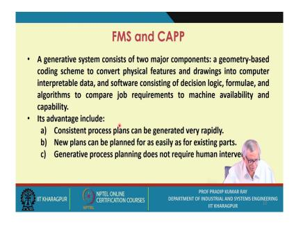
A generative system consists of two major components: a geometry-based coding scheme to convert physical features and drawings into computer interpretable data, and software consisting of decision logic, formulae, and algorithms to compare job requirements to machine availability and capability. Its advantage include:
