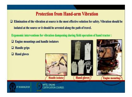
Now, some work we have also done with regard to the interventions (Refer Time: 30:25) and there we are talking of handle as isolators. These will also isolate the vibration from the hand from getting transmitted to the hand. The hand gloves have been found load, where various types of hand gloves are available.
