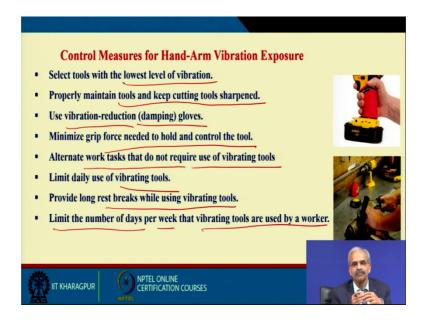
Control measures to hand-arm vibration exposure. There could be various control measures. Select tools with the lowest level of vibration. Properly maintained tools you keep cutting tools sharpened. These things may happen because many times we do exert pressure on them.
