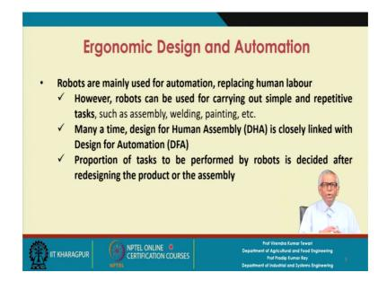
So, you use robots for automation. So, the robots are mainly used for automation replacing human labours. However, robots can be used for carrying out simple and repetitive task. such as assembly, welding, painting, etc.
