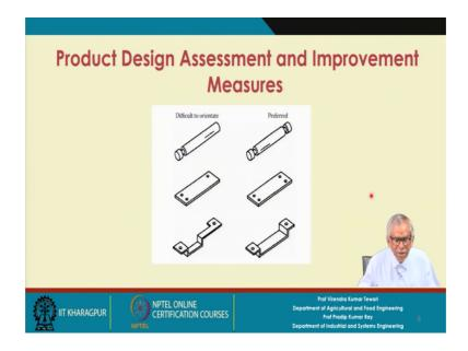
This is related to the symmetric parts. Now all the figure given in left side is asymmetric whereas all the figures in right side is symmetric. So, it will be very difficult to use the asymmetric parts for assembly.
