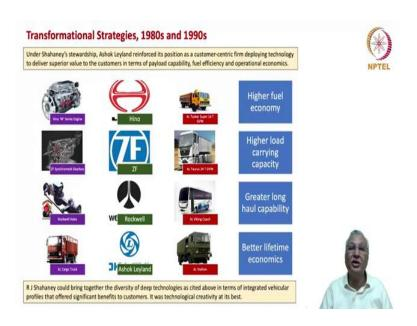
You can see some of the transformational strategies he adopted in 1980s and 1990s which I discussed. Hino W series engine which was available in 4 and 6 cylinder naturally aspirated turbocharged and turbocharged intercooled versions gave an unprecedented spread of horsepower from 60 horsepower to 220 horsepower that was very unique.
