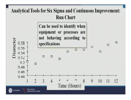
So, let say again you are making a wire right. So, first hour when you checked you just picked up one wire and you checked its diameter 0.5 centimeter right second hour you just pick one more wire diameter less than 0.5 and so on right. So, this how you will develop run chart right. So, you are measuring quality over period of time right.
