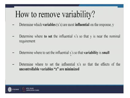
So, once you know which are the most influential variables, you need to set this influential variables in such a way that y is near near nominal requirement right. We should determine where to set the influential variable so that variability is small, this is our objective right and we want to set x variable in such a way that the effect of these z which are uncontrollable variable so, that effect is minimized right.
