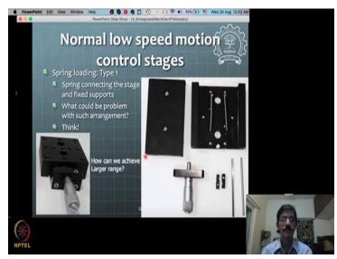
So, this is a screw here, screw has no, the threads are in this piece and then this is a screw and the screw has a small piece that is coming out and touching and pushing this upper stage, this is a upper stage. And you can see these two little springs here, the springs are tensioned and they are attached to this bottom piece, bottom piece is where this screw is assembled on the bottom piece here.
