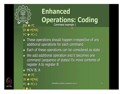
So, these are the operations that we said should happen. So, programme counter contents should go to memory address register and then whatever is addressed by that register to the memory, that location of the memory, contents of that location in the memory we transfer to IR register and then we update these, these are the, this is the sequence of operation should happen every single command that we execute. So, irrespective of any additional operations that are to be done.
