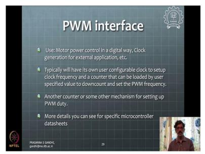
Now, we come to this PWM interface, which stands for pulse width modulation interface and this is very important interface for mechatronics engineers because this interface you can use for driving many different kinds of actuators or you can use it for cloud generation application for external peripherals. There are many different ways this interface can be used, but the most important is driving the actuators by this interface, why these interfaces used for driving actuators we will see that.
