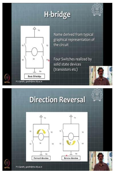
So, this H-bridge has a very simple way of switching the transistors and reversing the direction of the current in the motor. So, this is transistor-based switches are realized here. And this is one way direction and this is the other way direction reversal by switching S1 and S4 first and S3 and S2 the next or reversing the direction.
