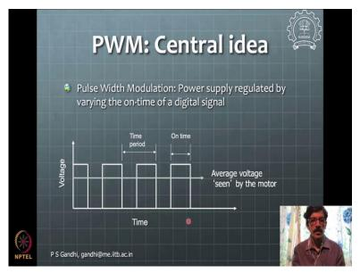
So, as I have told you, the pulse width modulation has this idea where the on-time period can be changed. So, now what happens when we do this thing going to the, to an amplifier the same kind of amplifier we use. So, we use same transistor amplifier, but now instead of giving analog as the input to that amplifier, we give this changing pulse as an input to the amplifier and this pulse is given at a very large frequency.
