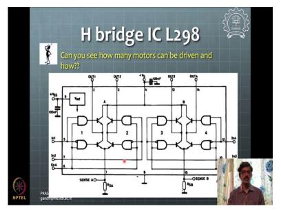
So, you can see this is a configuration of typical H-bridge. So, it has some gates to operate and things like that. And so, one can figure out from this block diagram of that chip, how this chip can be interfaced with your microcontroller and what to be, what is to be connected to motor to drive it. So, think about this, we will have this important exercise to be done.
