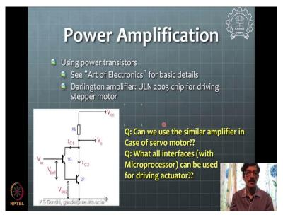
Suppose, we have a transistor-based amplifier. So, say ULN 2003 chip for driving stepper motor is there like that we are using some transistor amplifier. So, if we use this amplifier in the servo motor, so what we are talking here is right now, when we are talking in this actuator driver interface, we are typically the servo motor we are talking here not a stepper motor here and this servo motor not really this aero modelling servo motor.
