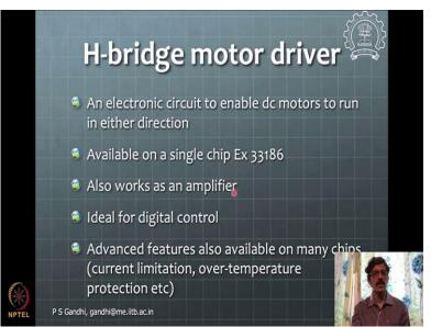
Then, how do we reverse the detection is using this H-bridge and H-bridge there are these lot of these different, different chips available for H-bridge functionality and it works as an amplifier and additional reversal both functions are done in one chip and this is very good, ideal thing for motor control digital control of the motor. And there are many advanced features could be available in other chips. (Refer Slide Time: 33:54)
