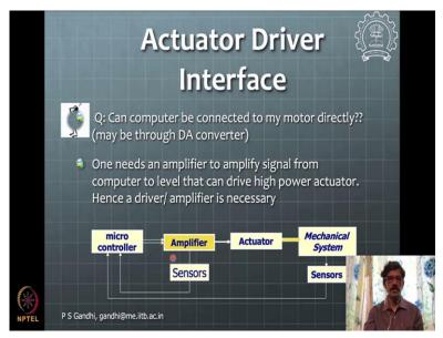
So, this now let us look at how this motor, why motor needs PWM interface. So, if you want to drive an actuator so, you need a driver for amplification. So, say because you cannot say I will connect my motor directly to my microcontroller and it will start running. No, imagine you cannot connect the ceiling fan, for example, to your microcontroller and expect it to run because the typically these motors will require larger power.
