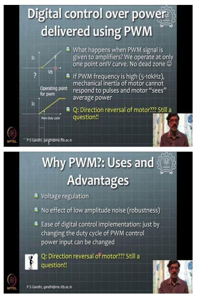
And suppose we give this input to our amplifier, then what happens is the value is always operated, operating point is always here because value is either 1 or 0 you can see that this value here is either 0 or 1. This is 1 here and this is 0 here. But only the period of on time it changed there is a time period and on time out of that is changed. So, since the on time is changed and this value is fixed, now this noise if you talk about that we said is in the small range here.
