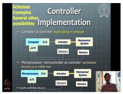
And these are like some of the schemes for implementation as we have seen these, one of these schemes we have seen already. You can have a computer or microprocessor or microcontroller, whatever you want to use for the brain or for the control of these. So, this is what is about interfacing different-different drivers and actuators here and we will see now how these interfaces can be then further used for building mechatronic application. Thank you.
