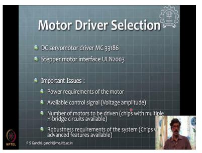
Then, there are many different drivers that can be possible for the, for this H-bridge or depending upon motor. So, permanent magnet DC motor can be driven by the H-bridge or a stepper motor can be driven by this some simple ULN transistor amplifier.
