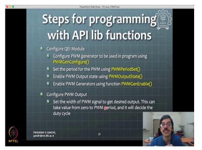
And then, so it is PWM generator configuration, so now we know what is PWM generator in the block. So, in that, you need to configure it PWM generator. So, it will typically have whether this will have a count up or count down, those kinds of things will be somewhere specified. These are QEI module. This is PWM all these are function for PWM modules.
