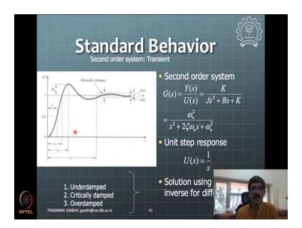
I am just flashing the same slides here actually. So, these are the standard first and second order system responses with this is this information should be handy to us for the application in several cases. And then we will have this formula for the second order system behavior formulae for maximum overshoot settling time this should be also handy to you.
