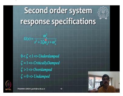
So, that as we saw in the pendulum problem for example we can use them to set up this omega n and  $\xi$  to have a desired value or when you do the pole placement problem the two dominant poles which you are placing close to the imaginary axis they can have some values taken by this thing.
