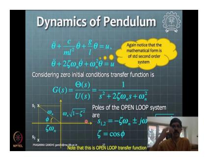
So, we come back to the system now we in the standard form it looks this and then can say write a transfer function of it. And then see the open loop poles are here then now we can propose some controller to move these poles around and things like that. So, that those are all kind of things can be done now.
