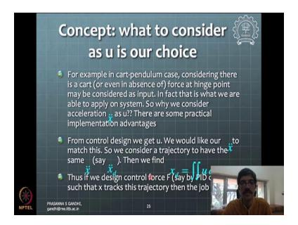
So, how do we do that now, so how do we... So, this is our control and control problem defined and suppose we find such a input u then how do we drive the cart such that this u is applied to pendulum that means we need to satisfy this equation. So, u is there and then  $x_{desired}$  now, this is not x here,  $x_{desired}$ , we can make it as  $x_{desired}$  here. So, my  $\ddot{x}_{desired}$  should be that u and I integrate this u twice with the scaling factor l.
