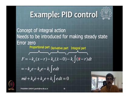
And the system has this steady state error you see there pause to the PD controller and you see that there is some kind of a steady state error then you introduce the integral control action. So, we will talk about this integral control action part I think this main kind of a thing or maybe we can give a summary of like when to use these different kind of control actions in generally in the system so this is be good to kind of know.
