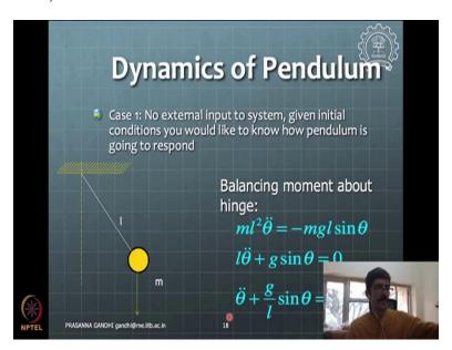
So, you can see this model of a pendulum here. So, this model is giving you this full nonlinear form of equation considering  $\Theta$  which is the angle of the pendulum here to be more than small angle approximation. So, with this model you can see that this has a harmonic kind of a behavior and that too without damping.
