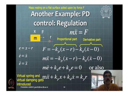
So, this is another example about the simple PD control for a regulation purpose. So, this is much simpler form which we have already seen. So, it is just again PD control applied here and you can
