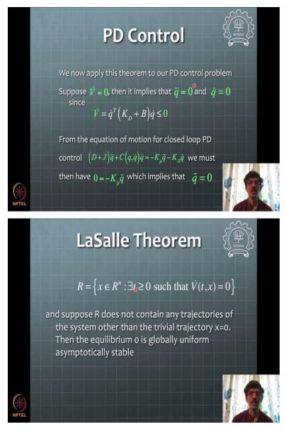
So, for PD Control we apply this theorem if we see that  $\dot{V}$  equal to 0 means  $\dot{V}$  is this. This = 0 that means  $\dot{q}$  equal to 0. Then  $\ddot{q}$  q when  $\dot{q} = 0$  I differentiate it once and I say that  $\ddot{q} = 0$ . And this is because it is  $\dot{q}$  equal not instantaneous it is for all time. So, we need to see that for all time t to 0  $\dot{V} = 0$  that is a condition that is coming.
