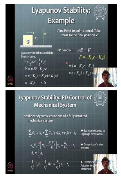
Now, we want to see that we propose this PD control on the joints. So,q is a generalized coordinate in terms of typically if it is a n degree of freedom robot then robot joints or generalized coordinate. So, in the direction of generalized coordinate you define this u where K p and K D are matrices they are kind of typically diagonal matrices. And  $\tilde{q}$  a is defined as q d minus q here.
