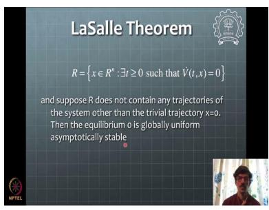
So we collect all such x together and observe them. And this such all these x or this set r does not contain any other trajectory of the system other than the trivial trajectory x equal to 0. Then the equilibrium x equal to 0 will be a globally uniformly asymptotically stable system. This is what is the LaSalle's theorem saying. So, this theorem is what we need to make use of in our case.
