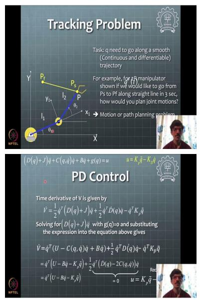
So, for that we need a lot more kind of thing to be done. So, the trajectory for tracking problem is simply like the suppose you have a tooling manipulator say I just explained by using this tooling manipulator. But we want to track this trajectory like say the problem is given that we will not like to go from Ps to Pf in three seconds along the along this path straight line path. This becomes like a motion or path planning problem.
