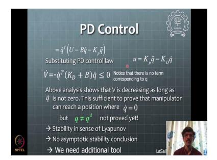
So, this LaSalle's theorem implies that then the system is asymptotically stable. And this is what like we make sure that our system is taken to the final position also. And final velocities are also to be desired value which is 0 the final position. Now, when the gravitational term is there then we need to compensate for that term. Because it is depend upon like the g (q) q means it is depend upon generalized coordinate that term can be computed and compensated for by the control.
