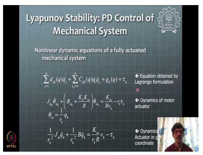
Now we can apply this to entire domain of this mechanical system so to say which are obtained by using our Lagrangian formulation applied to fully actuated mechanical system. Mechanical system I mean the rigid body mechanical system. We could restrict our discussion to rigid body systems alone here although some parts can be extended to flexible bodies also later but right right now for this course let us focus on only the rigid body systems multi body systems and fully actuated systems.
