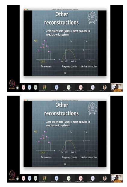
So, all that as not much of a physical value or implementation value in some sense; but it is just good to know that for this zero order hold; there is a the signal if it has triangle representation in a original frequency domain, analog signal; then it will get represented in some kind of a warp way, when it is sampled.
