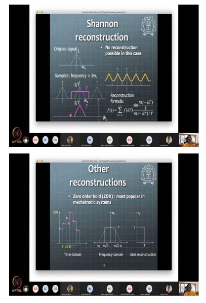
See, this is a sense that we talked about. The filter is filter in the frequency domain, allowing some signals to pass through; and some signals are completely not allowed to pass through. So, say when I say the filter is of this form, and like rectangle type form; then this particular filter function in the frequency domain, multiplies by frequency domain response to produce the output of the filter.
