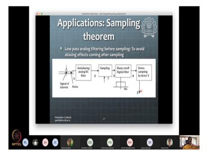
So, you have this signal of interest here is represented typically by our triangle representation. And then there is a void noise, which is our call frequencies; then you use this is called antialiasing filter. So, this analog domain RC filter is typically used, and then you can get the signal representation at the point 2.
