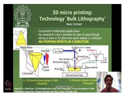
So, we thought we will do something different about it and then we started thinking that okay, what if we, what if we produce these components such that the photopolymer vat here has no layer, okay. So, that means this is complete volume here, it is complete volume production volume of the photopolymer is there and then we are, and then we are focusing the laser beam on the photopolymer at the, and the focus is matching with the bottom side of the substrate.
