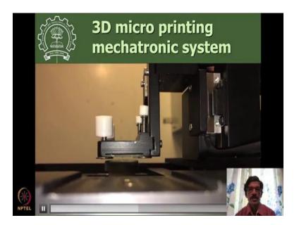
All these things are done in the software and then you put together all these in the system this is a dSPACE controller, then there are these voice call amplifiers in their power supplies and all these things are operating this system here, the voice coils are there inside and then this is a z stage. Now this z stage is stationary here is only some small adjustment if you want to do for focusing purposes the z stage will be moved.
