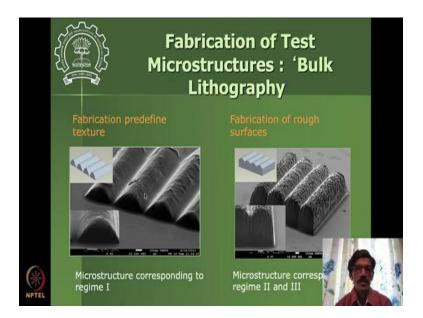
So, there are different-different micro structures fabricated by this process. And you can see that you know, at very small scale, we are able to do interesting structures possibility there are this lens array kind of structures here okay.
