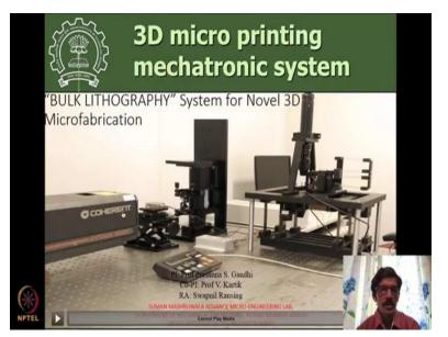
So, this is again we are using the same laser all other things are same. So, here is your coherent like the laser is there it is be steered by some optics and then it will be falling here on this cell system setup. And then you are going to kind of have the fabrication done by using some kind of motion of this XY stages in the compliant mechanism kind of way. And then there is this observer, the camera through which we can observe how things are getting fabricated and things like that, okay.
