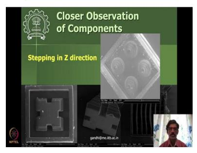
So, let us get started with this. So, if you see what we produced in the last study, micro printing technology is these components which are having this layered kind of structures, okay. So, these are at a macro scale, see, this is a 1 mm kind of distance here. So, in such a small kind of a distance you can print now various kind of components here, okay.
