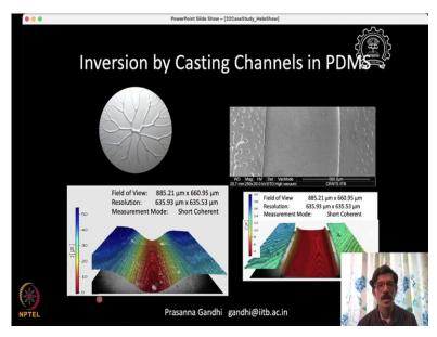
So, this these kind of patterns are very easy to get in this process and then we can invert is by casting in the material called PDMS is a kind of rubber kind of material in which these can be casted and then this can act as a micro channels. So, these things will have act as a micro channels of different cross sections.
