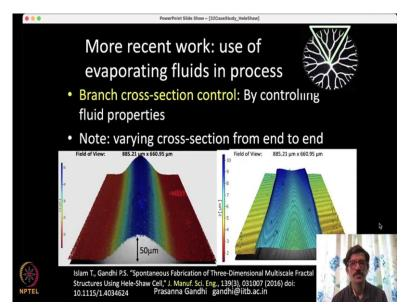
And one can explore this more I mean, when different different kinds of fluids you can have different possibilities. Say for example, if you use evaporating kind of liquid, evaporating solvent is evaporating, then you get these kind of patterns. So, this is a combination of liquid drying on the surface and this Hele-Shaw process.
