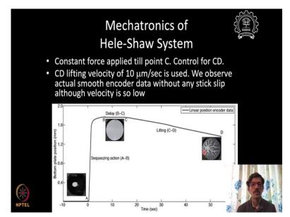
Then this we see the know the some of the results of the control. So, a control is done in a way that while squeezing we are squeezing from this point A to point B. So, this is a displacement or the plate position in mm kind of displacement of the point of the end. So, we are not plotting the angle here we are plotting the point of the motion of the actuator. Actuator moves the squeezing happens and like you will get this point here, this displacement of the endpoint here.
